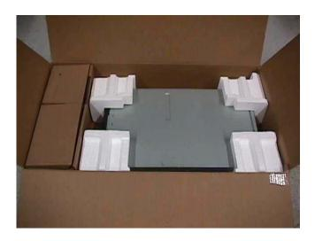
NOTE: Do NOT place extra shipgroup items in voids around the system. Materials placed in these areas will result in damage to the system.
