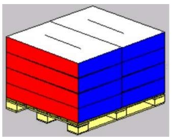
3.2.2 - Secure load to pallet (or half pallet) utilizing materials detailed out in Pkg BOM.
