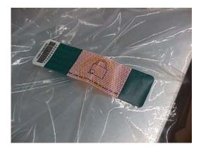
2.3 - Place cushions 25P1048 and 25P1049 onto the unit as shown. **Note: the bag is removed to show the unit orientation.**
