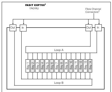
IN = primary or secondary (redundant) connection from FAStT700 Storage Server or previous FAStT EXP700 expansion unit daisy-chained from the storage server
