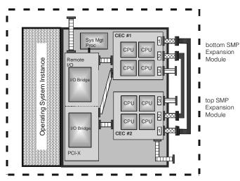
Logical Diagram of SMP Expansion Module cabling for 16-way x440 (two eight-way models) running one operating system. The top SMP Expansion Modules in each chassis are labeled CEC #2. Scalability ports are shown top to bottom one to three.
