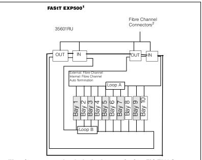
IN = primary or secondary (redundant) connection from FAStT500 Storage Server or previous FAStT EXP500 expansion unit daisy-chained from the
