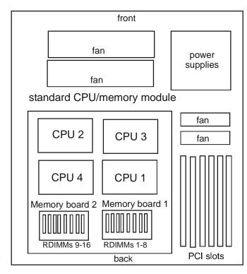
Optional SMP Expansion Module (P/N 59P5188) installs directly above standard CPU/memory board, requiring installation of four processors and a minimum of four RDIMMs. Standard with eight- and 16-way models.
