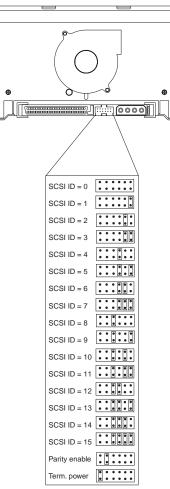
The default SCSI setting for the autoloader is 6. If you need to change the SCSI setting, refer to the SCSI ID settings shown in the illustration. To set the ID, remove and reposition the jumpers that come with your tape drive If necessary, use a pair of needle-nose pliers to remove the jumpers.
