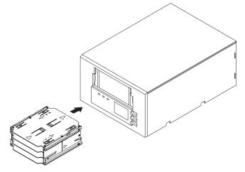
4. Gently push the magazine until the autoloader mechanism senses the magazine and pulls it into the autoloader.
