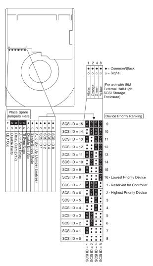
Assign SCSI ID 6, 5 or 4 to a IBM SCSI hard disk drive by placing jumpers on the drive as shown above. In most cases, you do not need to place jumpers on the drive's non-SCSI ID jumper pins.
