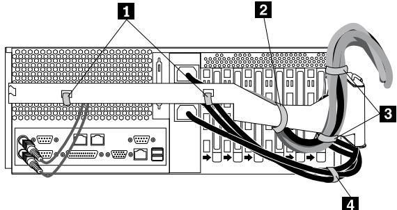
Use cable straps **1** to hold the cables in the cable-management arm. Secure the cables to the cable-management arm with a cable strap **2**. Route the cables under the right end of the arm; then, route them upward as shown and secure the cables with cable straps **3**. Secure the cables to each other as shown with cable straps **4**.
