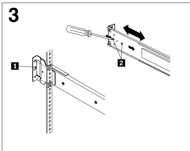
Use the tab **1** on the rear of the slide rail to align the slide rail to the rear of the rack cabinet. If it is necessary to adjust the length of the slide rail, loosen the screws **2** on the rear of the rail.
