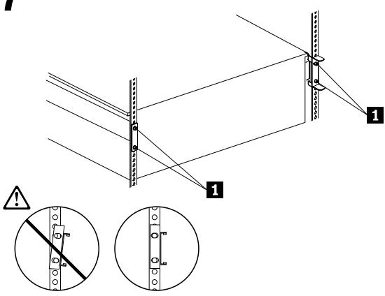
Press in on the slide-rail safety latches so that you can slide the server fully into the rack cabinet. Ensure that the rear slide-rail brackets are vertically aligned; then, fully tighten the rear M6 screws **1** on both slide rails.
