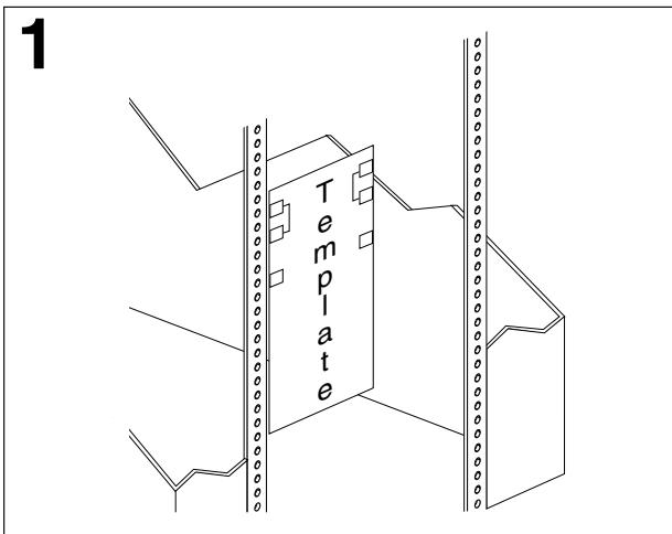
Use the attached stickers to mark the holes on the front and rear of the rack cabinet as indicated by the arrows on the attached rack mounting template.
