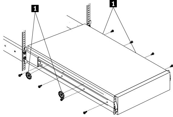
Use four M4 screws per side to secure the server to the rails; then, remove the rack-support wheels **1** and store them in a safe place.
