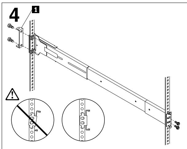
To install the left slide rail, ensure that the front slide-rail brackets are vertically aligned; then, insert and fully tighten both front M6 screws. Install the hinge bracket **1** before you insert the rear screws; then, partially tighten both rear M6 screws.
