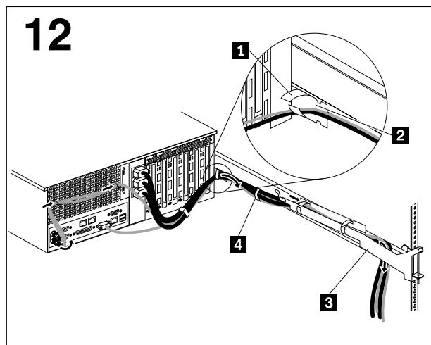
With the slide rails fully extended, attach the cables to the cable-retainer bracket **2**. Determine the length of cable needed between the server and the cable-management arm; then, route the cables through the cable-management arm **3**. Use cable straps to secure the cables to the bracket **1** and to each other **4**.
