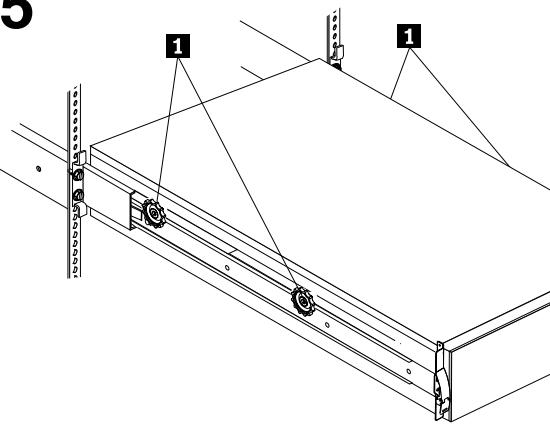
If you loosened the screws to adjust the length of the rail, tighten them now; then, fully extend the slide rails out of the rack cabinet until the slide rails lock into place.
