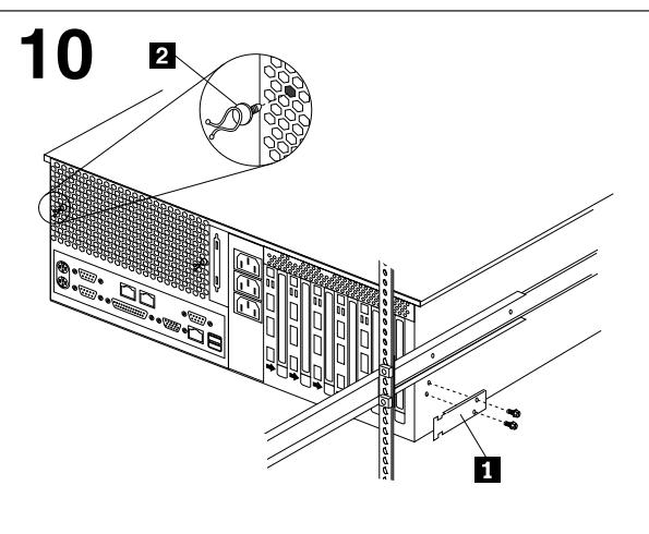
Use two M4 screws to install the cable-retainer bracket **1**; then, install the cable clamps **2** as shown.
