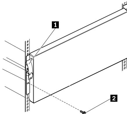
Slide the server into the rack cabinet until the release latches **1** lock into place.
