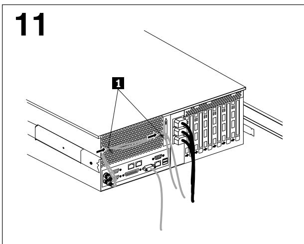
Attach the power, keyboard, mouse, and monitor cables (if required) to the rear of the server. Route the cables through the cable clamps **1**; then, attach all other required cables to the server.
