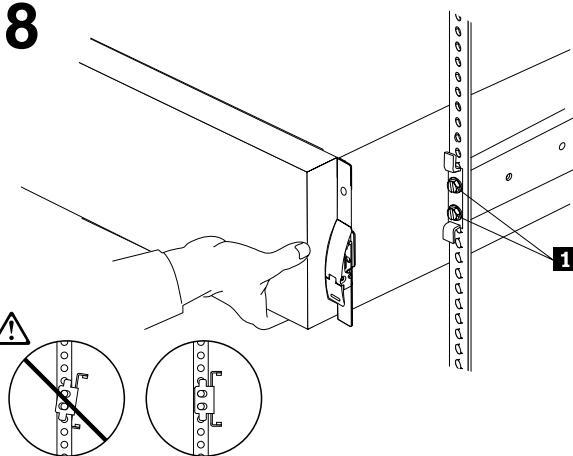
Slide the server halfway out of the rack cabinet; then, loosen but do not remove the front M6 screws **1** on both slide rails. While one person supports the front of the server by lifting it slightly, ensure that the slide-rail brackets are vertically aligned; then, fully tighten the front M6 screws on both slide rails.
