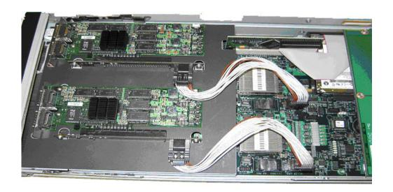
Figure 18. Overview with two InfiniBand options installed
