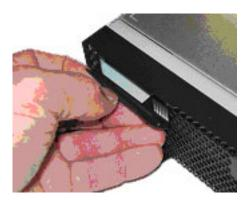
Figure 10. Removing the InfiniBand slot cover
