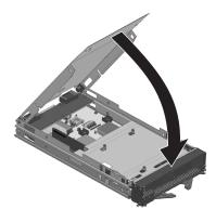
Figure 22. Closing the blade server cover
