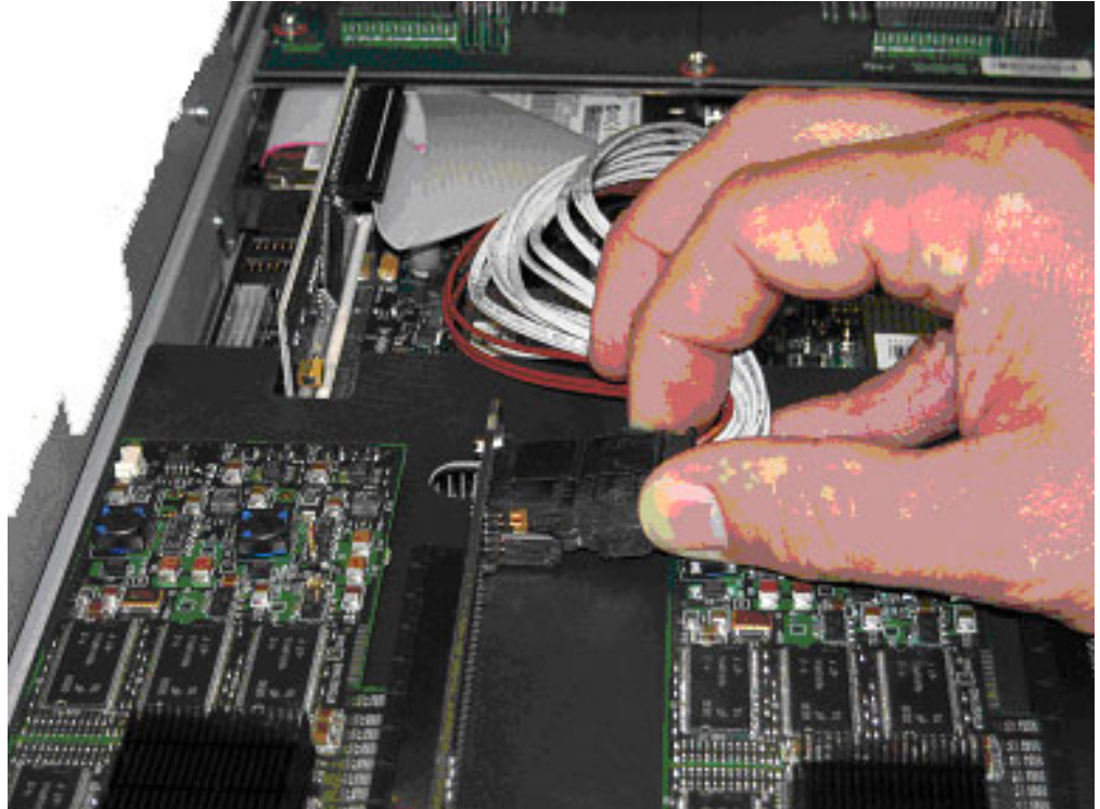
Figure 19. PCI Express connector installation (if you have installed the second InfiniBand option)
