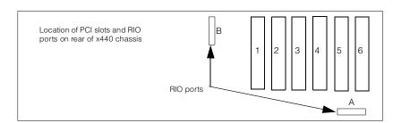
Slot 1: Bus A, 66MHz, 64-bit, full-length, 3.3v
