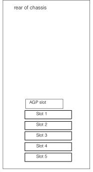
All PCI expansion slots are full-length, 32-bit, 33MHz, 5V or universal on a single PCI bus.
