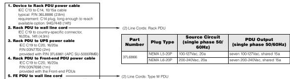
Part Source Circuit (50/ **PDU Output Plug Type** Number 60Hz) (single phase 50/60Hz) hree 100-127Vac. 20a each, shared 37L6883 NEMA L5-30P 100-127Vac, 30a, single-phase 200-240Vac, 30a, single phase 37L6884 NEMA L6-30P three 200-240Vac, shared 20a ne-to-line with ground 200-250Vac, 30a, three-phase three 100-127Vac (115-145), 20a NEMA L21-30P 37L6886 Y-connection with neutral
