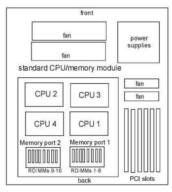
Optional SMP Expansion Module (P/N 32P8340) (installs directly above standard CPU/memory board). Ships prepopulated with four processors. Requires a minimum of four RDIMMs.
