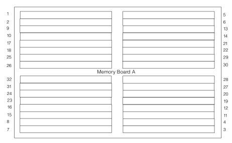
Install memory options according to the order shown for Memory Board A above. Repeat for Memory Board B.
