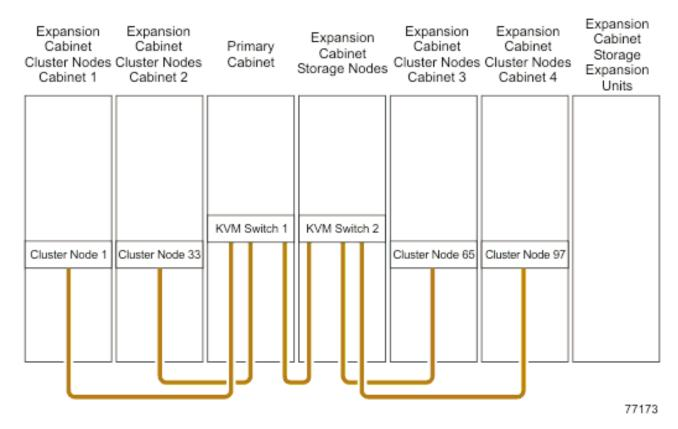
Figure 9. Intercabinet cabling for KVM connections
