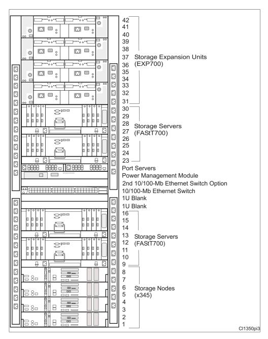
Figure 3. Example of an @server Cluster 1350 Expansion cabinet containing storage controllers and mass storage
