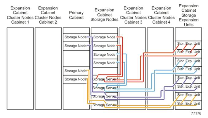
Figure 8. Intercabinet cabling for Fibre Channel connections.. To avoid making the Storage Node a single point of failure, connect two Storage Nodes to each Storage Server, as shown.
