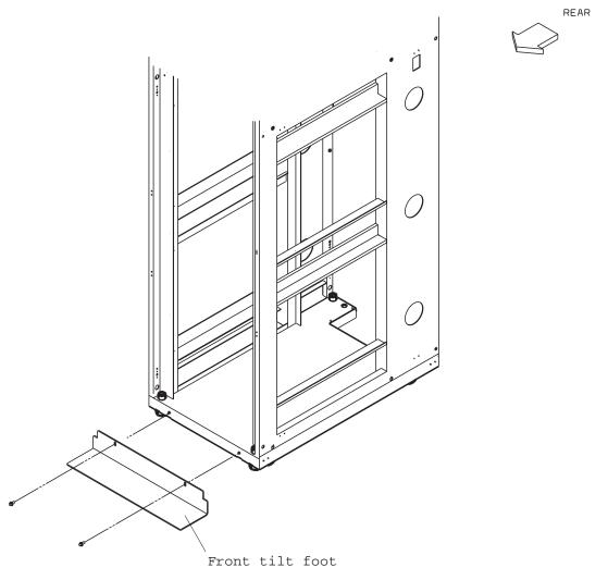
Figure 4. Frame stabilizer (tilt) foot installation
