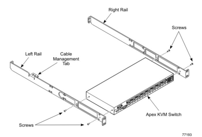
Figure 10. Mount switch rails to the console switch
