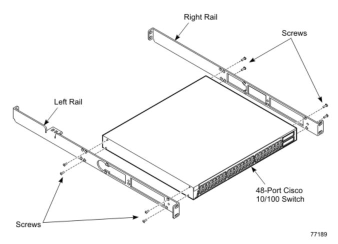
Figure 14. Mount switch rails to the Cisco 48-port 10/100 Switch
