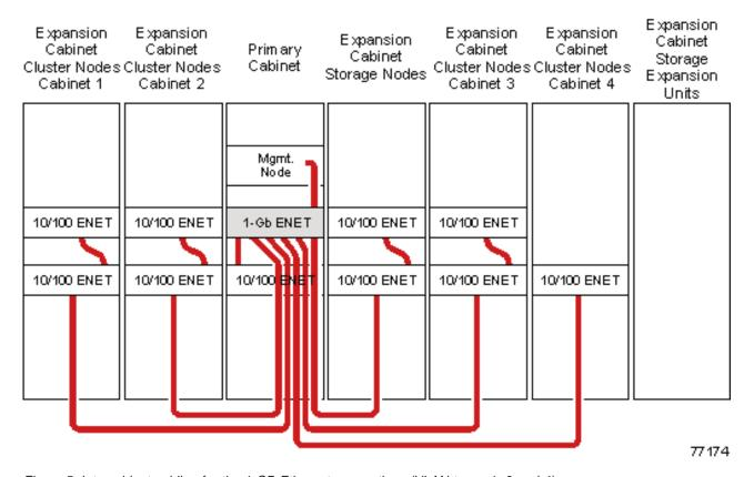
Figure 5. Intercabinet cabling for the 1-GB Ethernet connections (VLAN types 1, 3 and 4)
