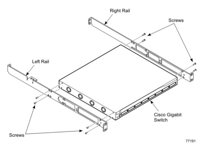
Figure 16. Mount switch rails to the Cisco Gigabit Switch
