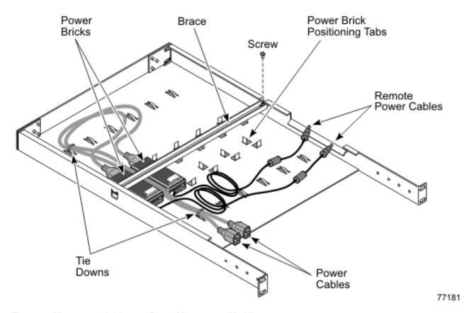
Figure 20. Mount power bricks onto Power Management Module tray
