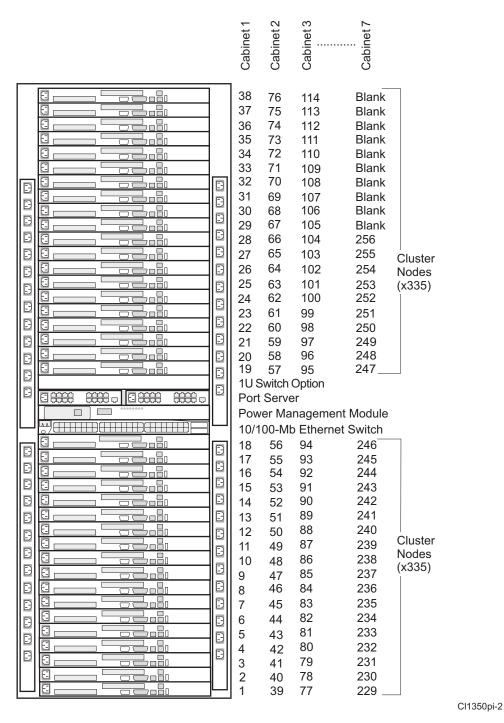
Figure 2. Example of an @server Cluster 1350 Expansion Cabinet with Cluster Nodes. This figure also shows how the node numbering scheme maps to other Expansion Cabinets.
