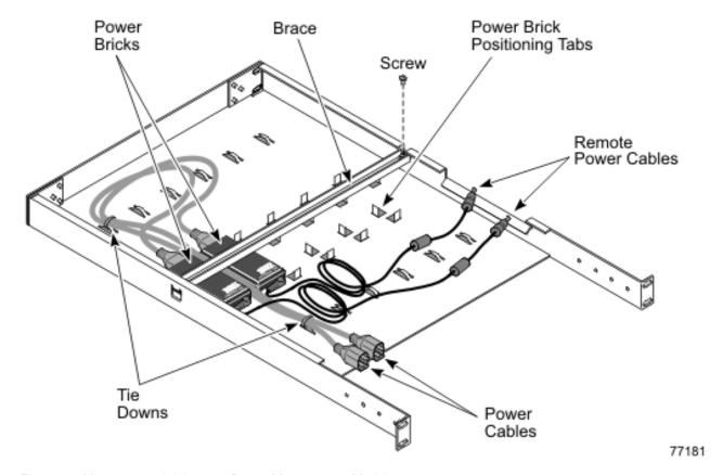
Figure 23. Mount power bricks onto Power Management Module tray
