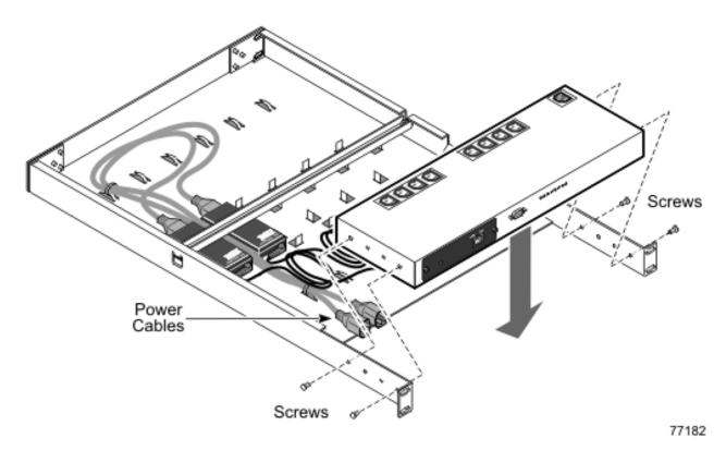
Figure 19. Mount Power Management Module onto Power Management Module tray
