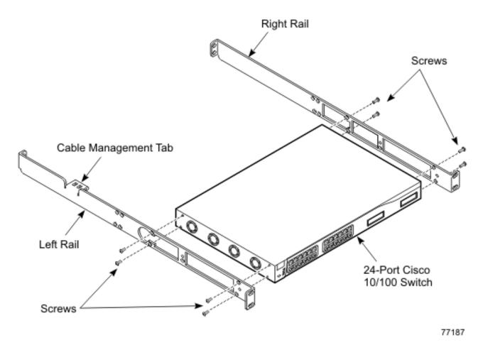
Figure 12. Mount switch rails to the Cisco 24-port 10/100 Switch
