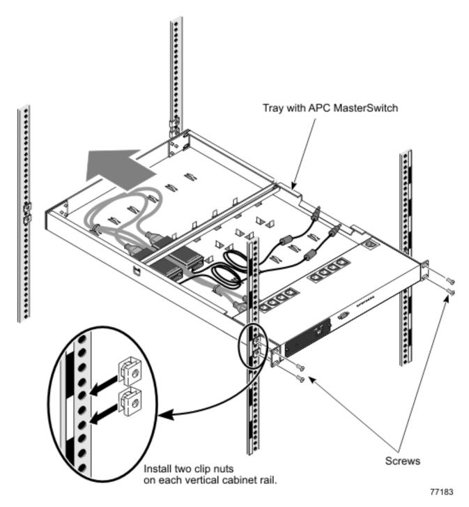
Figure 21. Install Power Management Module tray into cabinet from the rear of the cabinet, part 1
