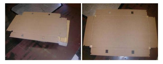
**2.4** Attach PBJ tray (22K8090) to pallet using a minimum of eight staples (22K8096) as shown.
