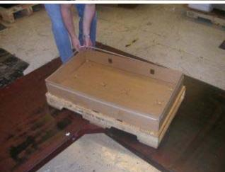
**2.6** Locate two universal fabricated cushions (22K8075) in preparation for placing in tray. Make sure they are set up correctly as shown below.
