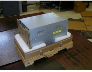
2.15 Locate PBJ carton (22K8186) and fold bottom panels into carton, ends first.
