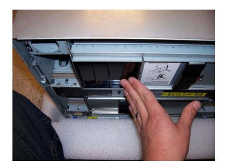
**2.14** Place assembled rear load spreader between rear face of system and rear cushion. Make sure the text is facing outward and upward and the tabs point toward the system.
