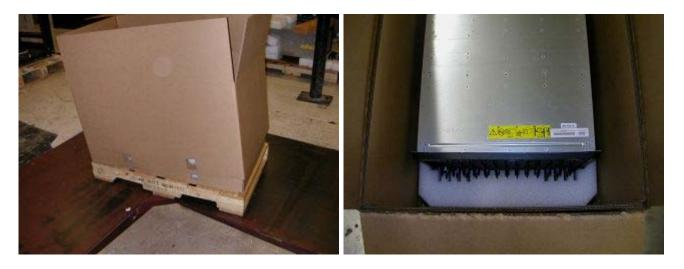
**2.17** Attach carton to tray/pallet assembly using four corrugated clips (37L0511).
