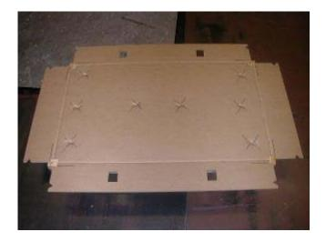
**2.5** Use Sanstrap (37L7558) to set up tray as shown below. The notches on each flap will help hold Sanstrap in place.
