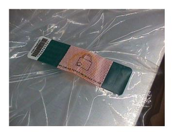
**2.11** After sealing the bag tape the unpack instructions to the top of the machine as shown below.
