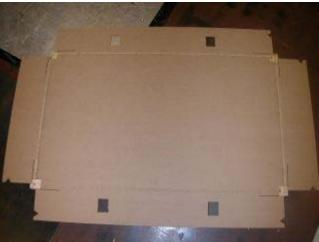
2.4 Attach PBJ tray (22K8090) to pallet using a minimum of eight staples (22K8096) as
