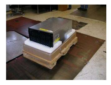
**2.10** Making sure bag is pulled tight, use Tamper Label (06P6550) to seal edges of bag closed.
