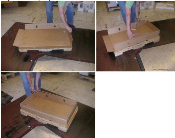
**2.6** Locate two universal fabricated cushions (22K8100) in preparation for placing in tray. Make sure they are set up correctly as shown below.
