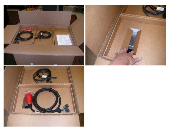
**2.21** Close the top of the carton and seal with printed tape. (74F5699 - Automatic taper, 74F5698 - for hand held dispensers).
