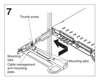
Align the cable-management-arm mounting plate with the rear of the server so that the four locking tabs on the mounting plate are aligned with the four tabs on the server. Slide the mounting plate to the left to engage the tabs; then, tighten the thumbscrew to secure the mounting plate to the server.
