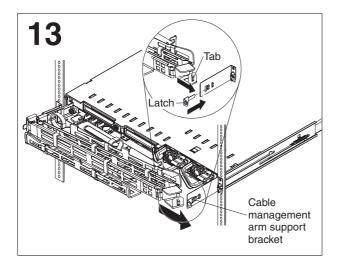
While you install and route cables, and before you ship the server, you must secure the free end of the cable-management arm. Insert the tab on the arm into the support bracket and then secure it by sliding the latch into place.
