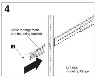
Attach the slide rail and the cable-management-arm mounting bracket to the left rear mounting flange with a single screw **1**. The screw should be only finger tight.
