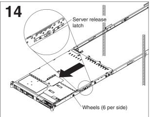
To remove the server from the rack, disconnect the cables and the cable-management arm from the server; then, slide the server forward until it latches in the service position. Press the server release latches on both sides of the server, and pull the server completely out of the slides.
