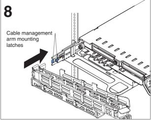
Align the cable-management arm with the two mounting latches. Slide the arm toward the server until both latches mate to their mounting brackets with audible clicks. To verify correct installation of the cable-management arm, extend the server fully from the front of the rack and verify that the arm moves freely. Push the server all the way back into the rack cabinet.
