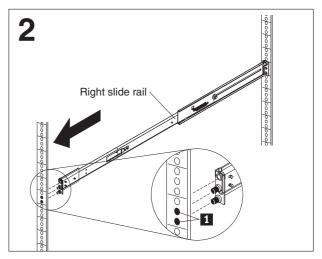
Extend the right slide rail and insert it into the front rack mounting flange, with the rail pins **1** protruding through the flange. Insert the left slide rail in the same way.
