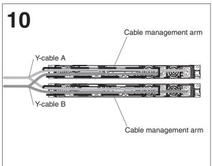
If you have installed a second ac power supply in each of the servers in the rack, you can use the Y power cable that came with the power-supply kit option to ensure server redundancy. Cable the servers as shown in the illustration, using one Y power cable to provide power to two different servers. Each Y power cable must be connected to a different power source, such as a power distribution unit (PDU), to maintain redundancy.
