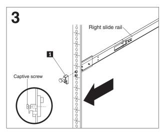
Attach one latch strike **1** to the front of the right rail, using the captive screw. The screw should be only finger tight. Attach the other latch strike to the front of the left rail in the same way.
