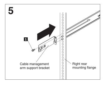
Attach the other slide rail and the cable-management-arm support bracket to the right rear mounting flange, using a single screw **1**. The screw should be only finger tight.
