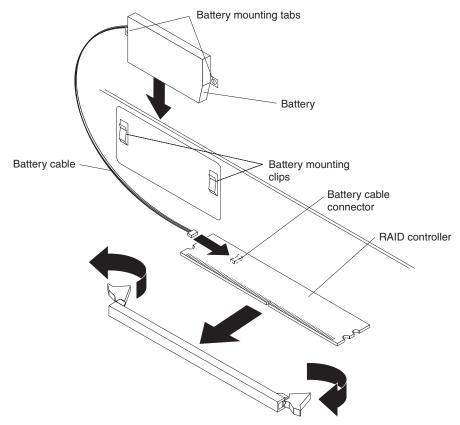
**Attention:** Incomplete insertion might cause damage to the server or the controller.
