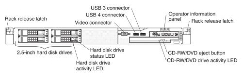
The following illustration shows the controls, LEDs, and connectors on the front of the server. This configuration supports up to two 3.5-inch hot-swappable hard disk drives or two 3.5-inch simple-swap SATA hard disk drives.
