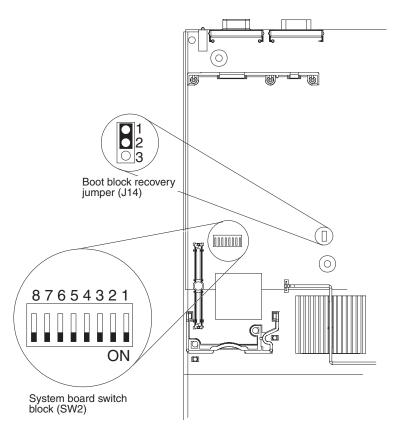
**Attention:** Before changing any switch settings or moving any jumpers, turn off the server; then, disconnect all power cords and external cables. See the safety information that begins on page v. Do not change settings or move jumpers on any system-board switch or jumper blocks that are not shown in this document.
