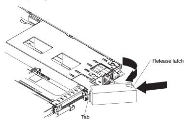
Press in on the release tab on the outside of the cover. Move the cover off the power supplies by swinging the cover to the left; then, remove it from the tab on the other side. Pull it back and off, and store it in a safe place.
