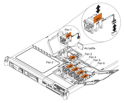
If you install a second microprocessor in the server, you must install one additional fan.
