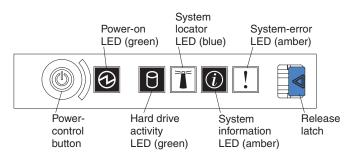
The following controls and LEDs are on the operator information panel:
