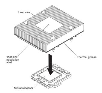
If you have to remove the heat sink after installing it, alternately loosen the screws to help break the bond between the components without damaging them.
