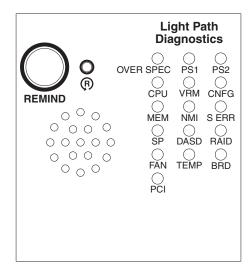
• **Remind button:** This button places the system-error LED on the front panel into Remind mode. In Remind mode, the system-error LED flashes rapidly until the problem is corrected, the system is restarted, or a new problem occurs.
