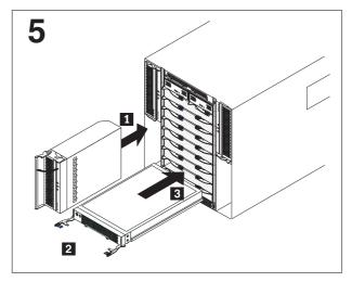
**Note:** If installing a preconfigured BladeCenter T unit, label the blade servers and BladeCenter T unit bays to ensure that you reinstall the blade servers in the intended bays. Reinstalling a blade server into a bay different from the one from which it was removed could have unintended consequences. Some configuration information and update options are established according to bay number.
