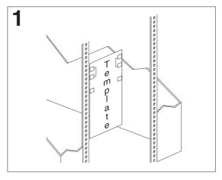
Position the template on the rack so that the edges of the template do not overlap any other devices to be installed. Line up and select the holes on the front and rear of the rack in the locations indicated by the arrows on the attached template.
