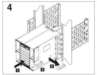
Carefully lift and place the rear edge of the unit on the front shelf brackets. Slide the unit along the shelf brackets until the rear lift handles are close to the front brackets 1.
