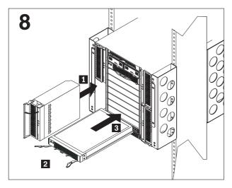
Carefully reinstall the power modules **1**, blade servers **3**, and bezel assembly in the BladeCenter T unit. (See the *BladeCenter T Types 8720 and 8730 Installation and User's Guide* for installation procedures.)
