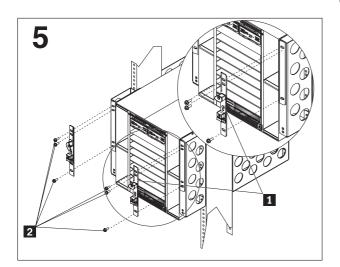
Align the holes in the bezel lock bracket **1** with the holes in the mounting bracket; then, secure the bezel lock and mounting bracket to the shelf bracket with three M6 combination-head screws
