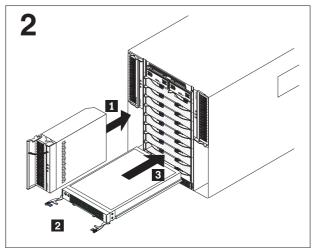
**Note:** If installing a preconfigured BladeCenter T unit, label the blade servers and BladeCenter T unit bays to ensure that you reinstall the blade servers in the intended bays. Reinstalling a blade server into a bay different from the one from which it was removed could have unintended consequences. Some configuration information and update options are established according to bay number.
