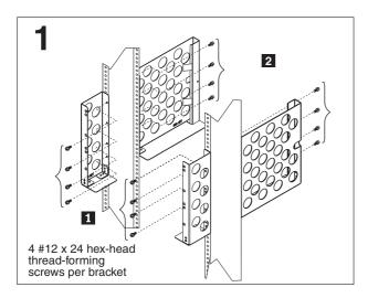
Align the front shelf bracket to the rack flange. Attach the front shelf bracket to the rack flange by installing four #12-24 hex-head thread-forming screws 1 into the rear of the bracket.
