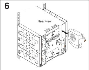
Reinstall the blowers in the BladeCenter T unit. (See the *BladeCenter T Types 8720 and 8730 Installation and User's Guide* for installation procedures.)
