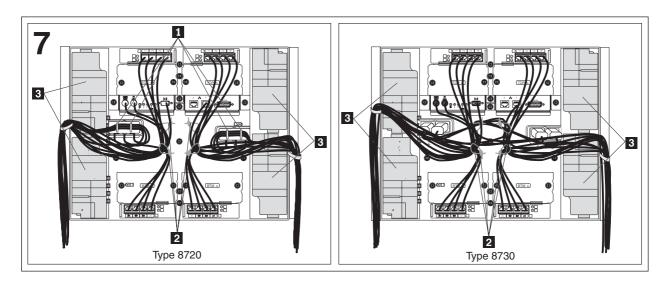
Attach the power cords and other cables to the rear of the BladeCenter T unit. (For details about connecting the dc-power cables, see the *BladeCenter T Types 8720 and 8730 Installation and User's Guide.*) If installing Type 8720, route the power cables through the cable ties on the dc-power cover 1; then, route all the cables as shown in the illustration.
