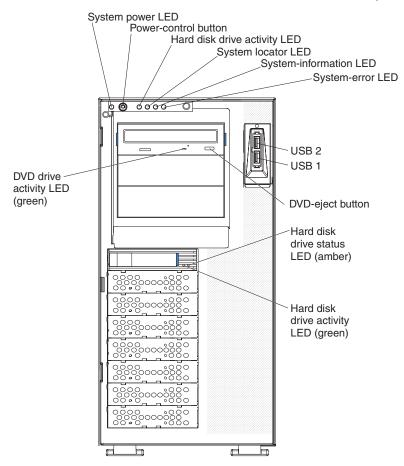
**System Power LED:** When this LED is lit and not flashing, it indicates that the server is turned on. When this LED is flashing, it indicates that the server is turned off and is still connected to an ac power source. When this LED is off, it indicates that ac power is not present, or the power supply or the LED itself has failed. A power LED is also on the rear of the server.
