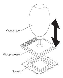
1) Squeeze and hold the bladder of the tool; then, place the suction cup on the microprocessor and release the bladder.
