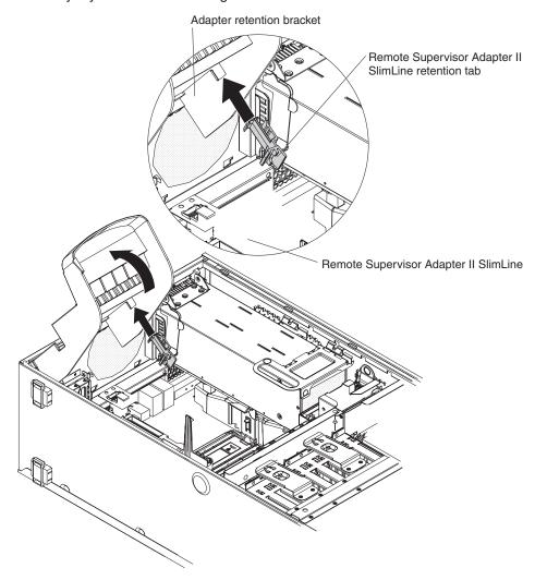
Open the rear adapter retention bracket and install the Remote Supervisor
