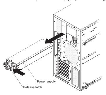
9. Remove the power-supply and power supply filler from the server by pressing down on the release latch while you pull out.
