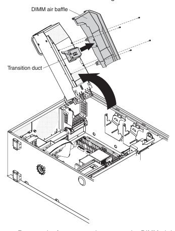
a. Remove the four screws that secure the DIMM air baffle to the power-supply cage.
