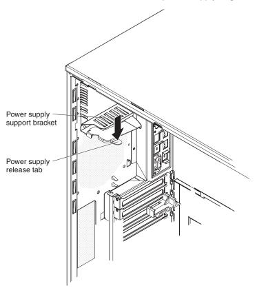
13. Raise the power-supply cage slightly and press and hold the release tab on the rear power-supply support bracket; then, lower the power-supply structure into position. The power-supply cage is not shown in the illustration for clarity.
