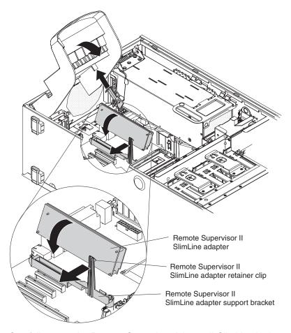
Carefully grasp the Remote Supervisor Adapter II SlimLine by its top edge or upper corners, and align it with the Remote Supervisor Adapter II SlimLine guide and the connector on the system board.
