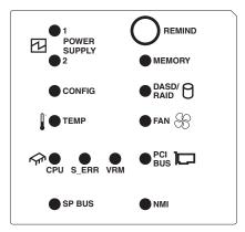
Press the remind button on the light path diagnostics panel to acknowledge an error has occurred but indicates that you will not take immediate action. When you press the remind button, the system-error LED flashes every 2 seconds until the error is corrected. If another error occurs, the system-error LED stops flashing and is lit again.
