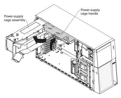
5. Lift the power-supply cage handle on the rear of the power supply cage, and rotate the power-supply cage out of the way until it latches in place. Let the power-supply cage rest on the rear power-supply structure support bracket.
