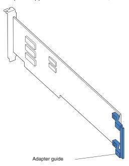
7. Press the adapter *firmly* into the expansion slot, lower the adapter retention brackets, and make sure that the brackets are closed. To release the rear adapter retention bracket press up on the retention clip while rotating the bracket forward.
