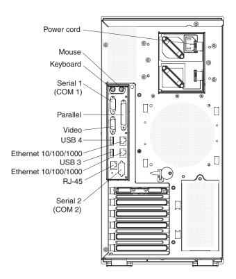
**Power-cord connector:** Connect the power cord to this connector.
