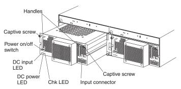
Handle: Use the two handles for installing and removing the power supply.
