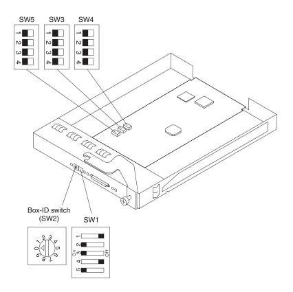
**Note:** If both ESMs are installed, the ESM on the left must have valid switch settings. The switch settings on the ESM that is installed in the right bay are ignored. If only one ESM is installed, it must be in the left bay.
