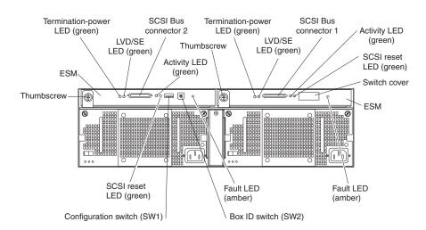
**ESM** Each ESM contain SCSI controls, LEDs, and connectors.
