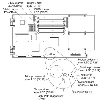
4. Press and hold the light path diagnostics button (SW1) to light the LEDs that were lit before you removed the blade server from the BladeCenter unit. The LEDs will remain lit for as long as you press the button, up to a maximum of 25 seconds.
