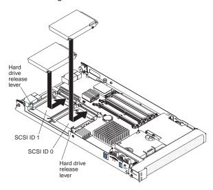
Note: Do not install a SCSI hard disk drive in SCSI connector 1 (SCSI ID 1) if you intend to also install an optional standard expansion card. The standard expansion card occupies the same area as the second drive.
