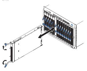
The following illustration shows how to install the blade server into a BladeCenter T unit.
