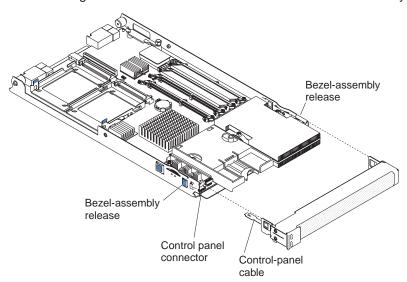
Complete the following steps to remove the blade server bezel assembly:
