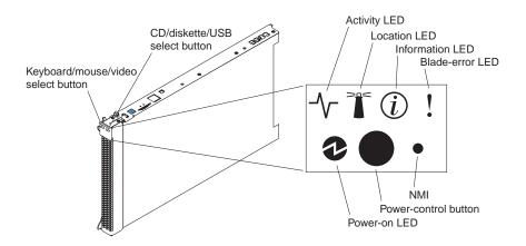
**Keyboard/mouse/video (KVM) select button:** Press this button to associate the keyboard port, mouse port, and video port with the blade server. The LED on this button flashes while the request is being processed then is lit when the ownership of the keyboard, mouse, and video has been transferred to the blade server. It can take approximately 20 seconds to switch the keyboard, video, and mouse control to the blade server.
