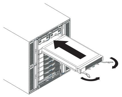
Complete the following steps to install a blade server in a BladeCenter unit.
