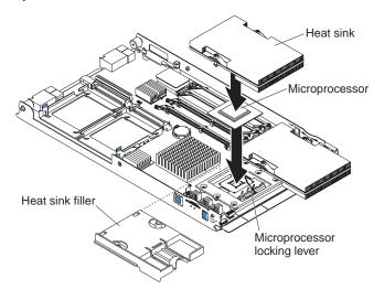
Complete the following steps to install an additional microprocessor:
