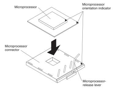
11. Close the microprocessor-release lever to secure the microprocessor.
