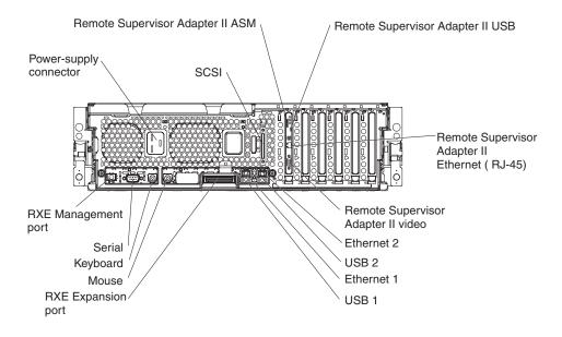
The following illustration shows the I/O connectors on the rear of the server.
