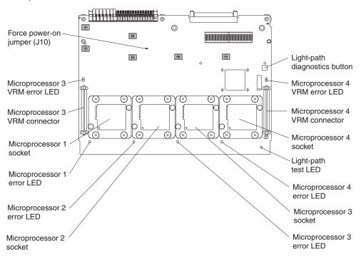
The microprocessor board contains the force power-on jumper (J10), a two-pin jumper block. The default is no jumper installed over the two pins. Place a jumper over the two pins to force the server to start up when you connect the server to ac power.
