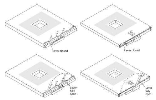
**Attention:** You must ensure that the locking lever on the microprocessor socket is in the fully-open position before you insert the microprocessor in the socket. Failure to do so might result in permanent damage to the microprocessor, microprocessor socket, and microprocessor-tray assembly.
