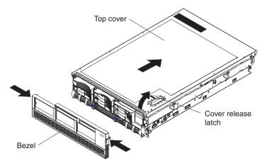
4. Lift the cover-release latch. The cover slides to the rear approximately 13 mm (0.5 inch). Lift the cover off the server.
