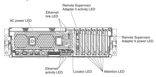
The following illustration shows the LEDs on the rear of the server.
