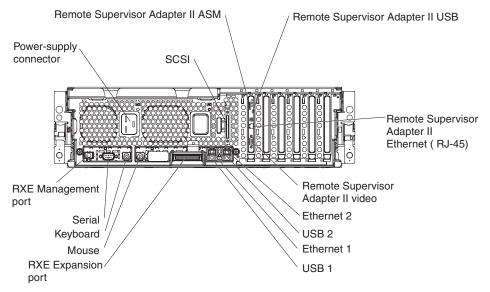
**Remote Supervisor Adapter II ASM connector:** Attach an ASM breakout cable to this connector to enable system management through the serial connectors and through the ASM RS-485 connectors.
