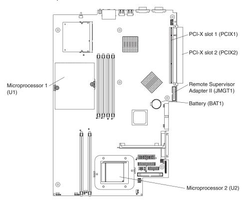
**Note:** The VRMs for the microprocessors are integrated on the system board.
