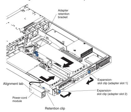
**Attention:** Avoid touching the components and gold-edge connectors on the adapter. Ensure that the adapter is completely and correctly seated in the slot. Incomplete insertion might cause damage to the system board or to the adapter.
