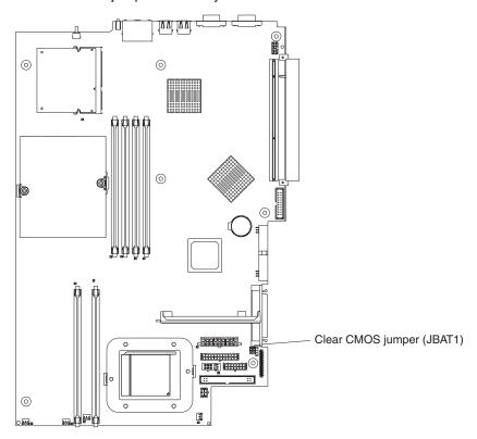
6. Change the position of the jumper on JBAT1 to bypass the password check.
