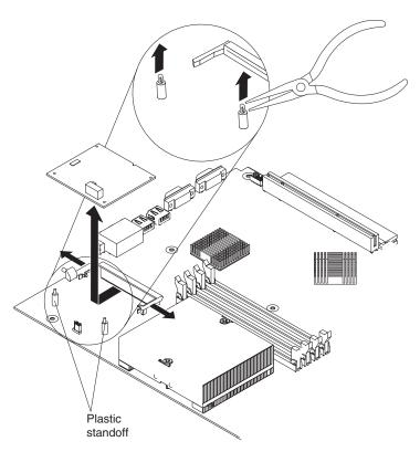
8. Gently pull up on the baseboard management controller until it disengages from the plastic standoffs. If the standoffs come away from the system board with the baseboard management controller, gently pull them out of the baseboard management controller and push them back into their apertures on the system board.
