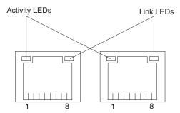
Connect Category 3, 4, or 5 unshielded twisted-pair cables to these connectors. The 100BASE-TX and 1000BASE-T Fast Ethernet standards require Category 5 or higher cabling.
