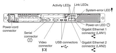
**Power-cord connector:** Connect the power cord to this connector.
