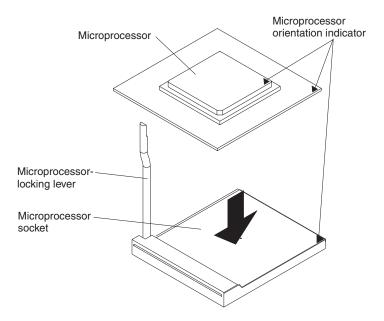
6. Close the microprocessor-locking lever to secure the microprocessor.
