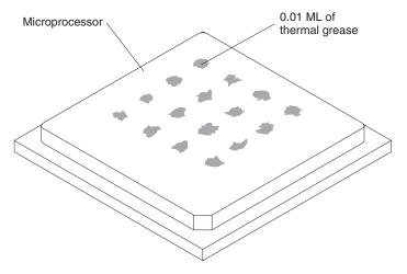
5. Use the thermal-grease syringe to place 16 uniformly spaced dots of 0.01 mL each on the top of the microprocessor.
