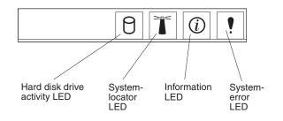
The following LEDs are on the operator information panel:
