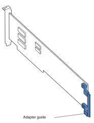
**Attention:** Be certain that the adapter is correctly seated in the expansion slot before you turn on the server. Incomplete installation of an adapter might damage the system board or the adapter.
