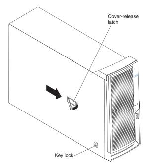
For hot-swap hard disk drive models, open the server door and hold the hot-swap lock bar in the closed position, lock the side cover key lock, and close the server door.
