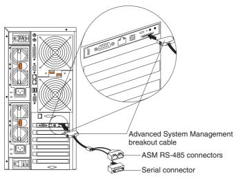
To connect the Remote Supervisor Adapter II to an ASM interconnect network, connect a Category 3 or Category 5 cable to one of the ASM RS-485 connectors on the ASM breakout cable. For more information, see Chapter 3, "Using the ASM interconnect network," on page 27.
