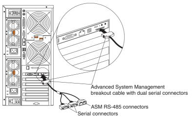
The ASM breakout cable with dual serial connectors also connects the Remote Supervisor Adapter II to the ASM interconnect network through the ASM RS-485 connector or to a modem through the serial connector.
