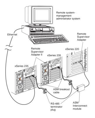
In the following example, a Remote Supervisor Adapter is installed in an xSeries 235 server and creates an interconnect network with the xSeries 235 server and the xSeries 350 servers. A modem is connected to the serial connector of the Remote Supervisor Adapter II (on one end of the ASM breakout cable), a modem is connected to the ASM PCI adapter in the server connected to the end of the ASM interconnect network, and a modem is connected to the remote system-management administrator's system.
