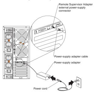
The following illustration shows the location of the power-supply connector on a Remote Supervisor Adapter II installed in a rack-mounted server.
