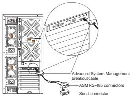
To connect the Remote Supervisor Adapter II to an ASM interconnect network, connect a Category 3 or Category 5 cable to one of the ASM RS-485 connectors on the ASM breakout cable. For more information, see Chapter 3, "Using the ASM interconnect network", on page 21.
