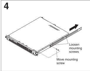
If you plan to transport the rack cabinet to another location with the server installed, remove one screw and loosen the other screws as indicated. Then, fully extend the rail and reinsert the screw and tighten all screws to secure the rail. Repeat this step for the other rail.
