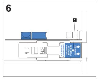
Press on the release tab **1** as indicated on the shipping bracket, and remove the shipping bracket from the slide rail. Repeat this step for the other shipping bracket. Store the shipping brackets for future use.
