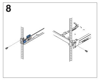
Before you transport the rack cabinet to another location with the server installed, you must secure the server to the rack. If necessary, disconnect the cables from the rear of the server; then, slide the server out of the rack 150 mm (6 inches) and insert the M6 screws in each slide rail. Then, secure the server to the rack cabinet with the M6 screws.
