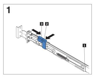
Press on the rail-adjustment bracket 1 on the rear of the slide rail to prevent the bracket from moving. Then, press on tab 2 and tab 3 and slide the rail-locking carrier toward the front of the slide rail until it snaps into place. Press on tab 2 and tab 3 on the front rail-locking carrier and slide the rail-locking carrier toward the rear of the slide until it snaps into place.
