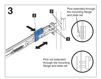
Align the pins 1 on the front rail-locking carrier to the front mounting flange. If you adjusted the rail length, push the rail-locking carrier back toward the rear of the slide rail to align the slide rail with the mounting flange 3. Then, press the tab 2 to secure the front of the slide rail to the front mounting flange.
