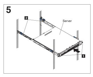
Align the server on the slide rails and push the server fully into the rack cabinet. Secure the server to the front mounting flanges with the captive thumbscrews 1.
