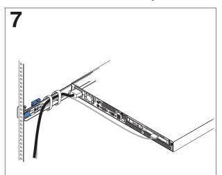
Attach cables to the rear of the server (such as keyboard, mouse, and monitor cables, if required). Route the cables to the left corner of the server (as viewed from the rear) and use the cable straps to secure the cables to the slide rails.
