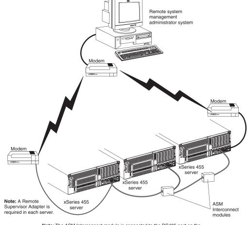
**Note:** The ASM Interconnect module is connected to the RS485 port on the back panel of the Remote Supervisor Adapter in each server.
