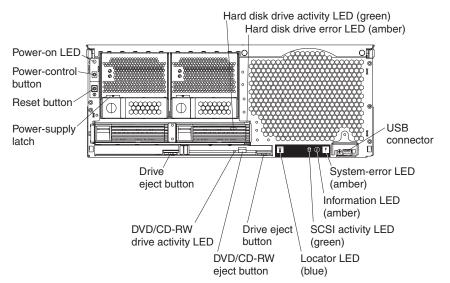
**Power-on LED:** When this LED is lit and not flashing, it indicates that the server is turned on. When this LED is flashing, it indicates that the server is turned off and still connected to an ac power source. When this LED is off, it indicates that ac power is not present.
