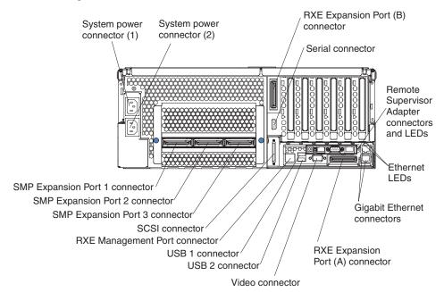
System power connectors (1 and 2): Connect the power cords to these two connectors to provide power to the server.
