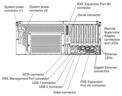
**System power connectors (1 and 2):** Connect the power cords to these two connectors to provide power to the server.
