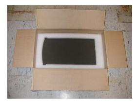
1.6- The Blade is placed into the middle of the PE Cushion 22K8230 with the Bezel facing curved section of cushion.
