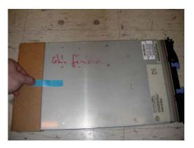
1.3- Place the Blade in ESD bag 37L8109, as shown below, and seal it closed using ESD label 6937292.
