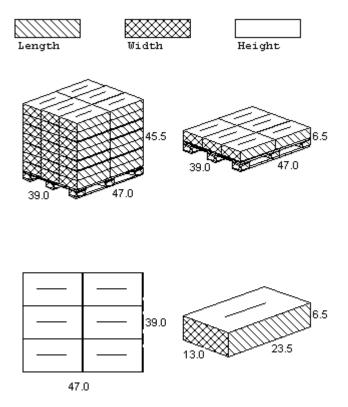
2.1.2 - Secure load to pallet utilizing "Best of Breed" palletization methods. See 92F6168 - "Best of Breed" Pallet Unitization or QMX document P-04146.
