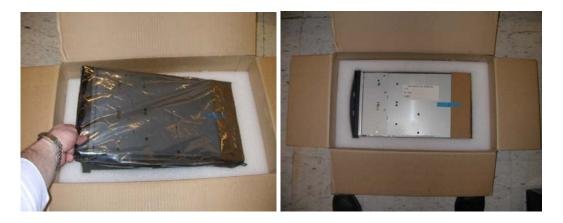
1.7- Remaining Urethane Cushion 22K8229 is placed on top of Blade. Top U-Tray 22K8231 is set on top of Cushion.
