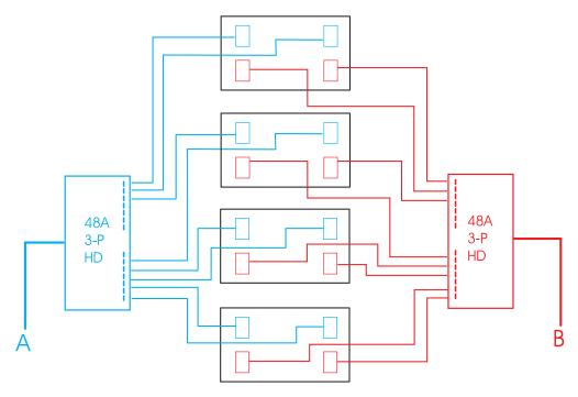
Figure 29. Power layout for four BladeCenter units in a NetBAY 42U rack with 1400 W power supplies (3-phase)
