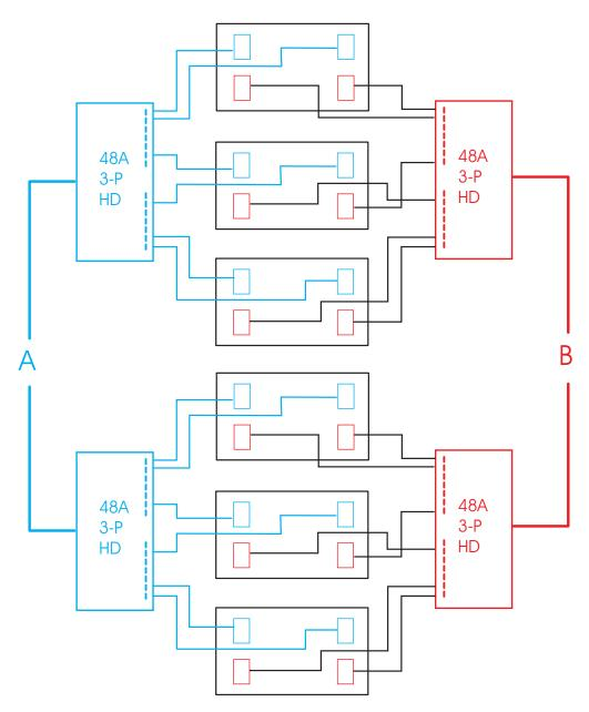
Figure 37. Power layout for six BladeCenter units in a NetBAY 42U rack with 1200 or 1400 W power supplies (3-phase)
