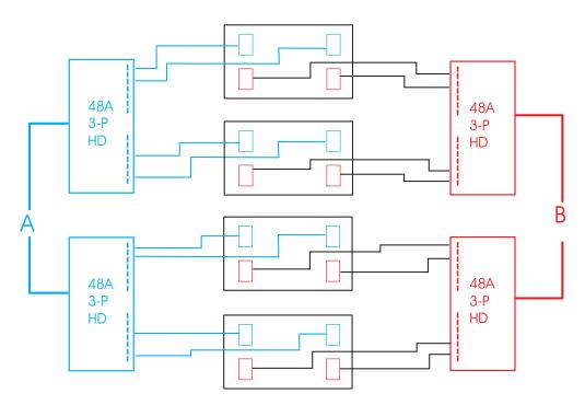
Figure 30. Power layout for four BladeCenter units in a NetBAY 42U rack with 1400 or 1800 W power supplies (3-phase)
