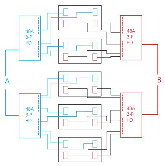
Figure 34. Power layout for five BladeCenter units in a NetBAY 42 rack with 1400 and 1800 W power supplies (3-phase)
