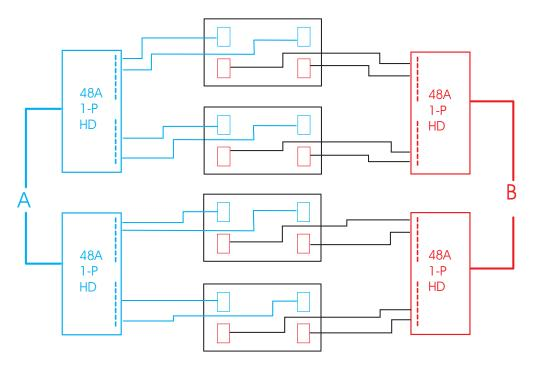
Figure 28. Power layout for four BladeCenter units in a NetBAY 42U rack with 1400 or 1800 W power supplies
