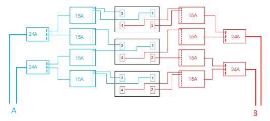
Figure 22. Three BladeCenter units in a NetBAY 25 or 42 rack; 1200 W power supplies
