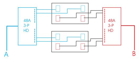
Figure 21. Power layout of two BladeCenter units installed in NetBAY 25 to 42U racks with 1400 or 1800 W power supplies (3-phase)
