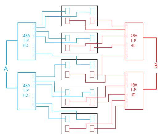
Figure 33. Power layout for five BladeCenter units in a NetBAY 42 rack with 1400 W power supplies
