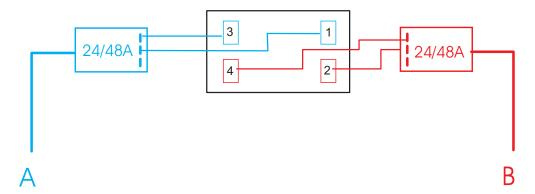
Figure 16. Power layout of a single BladeCenter installed in a NetBAY 25 or 42U rack with jumper cable
