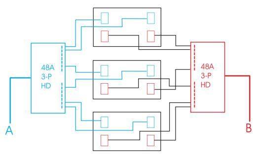
Figure 25. Power layout for three BladeCenter units in a NetBAY 42U rack with 1400 or 1800 W power supplies (3-phase)
