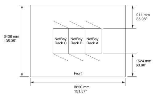
Figure 9. Operational clearances for NetBAY 42 Enterprise rack
