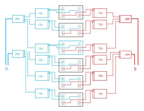
Figure 35. Six BladeCenter units in a NetBAY 42U rack; 1200 W power supplies
