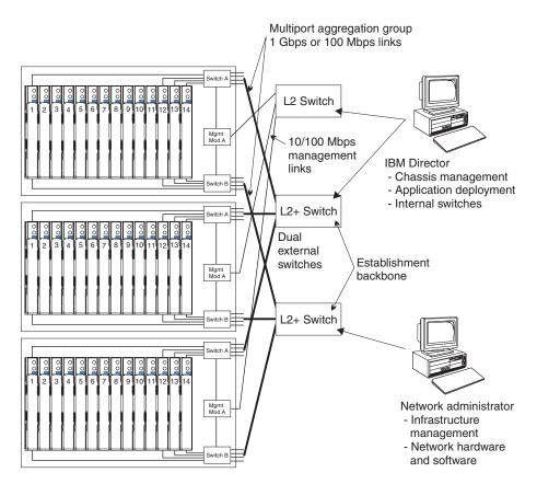
Figure 44. Recommended network topology with multi-port link aggregation groups
