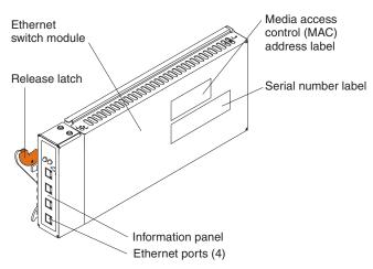
This section provides a summary of the features for your IBM xSeries<sup>™</sup> 4-Port Gb Ethernet Switch Module.
