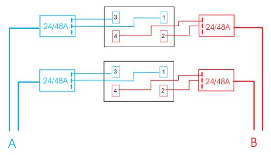
Figure 19. Two BladeCenter units installed in NetBAY 25 to 42U racks with jumper cable
