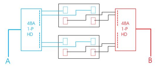
Figure 20. Power layout of two BladeCenter units installed in NetBAY 25 to 42U racks with 1400 or 1800 W power supplies
