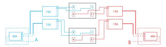
Figure 18. Two BladeCenter units installed in NetBAY 25 to 42U racks; 1200 W power supplies
