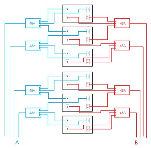
Figure 36. Six BladeCenter units in a NetBAY 42U rack; 1400 or 1800 W power supplies
