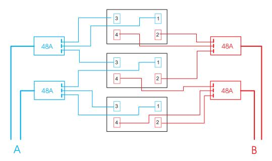
Figure 24. Three BladeCenter units in a NetBAY 25 or 42 rack; 1400 or 1800 W power supplies
