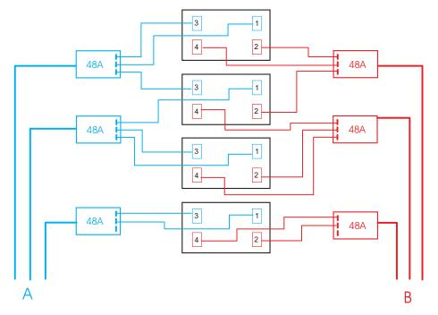
Figure 27. Four BladeCenter units in a NetBAY 42U rack; 1400 or 1800 W power supplies
