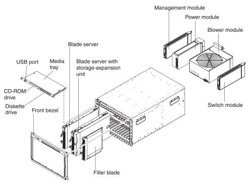
**Attention:** To maintain proper system cooling, each module bay must contain either a module or a filler module, and each blade bay must contain either a blade or a filler blade.
