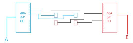
Figure 17. Power layout of a single BladeCenter installed in a NetBAY 25 or 42U rack with 1400 or 1800 W power supplies (3-phase)
