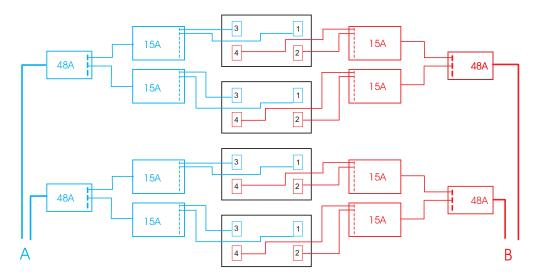
Figure 26. Four BladeCenter units in a NetBAY 42U rack; 1200 W power supplies
