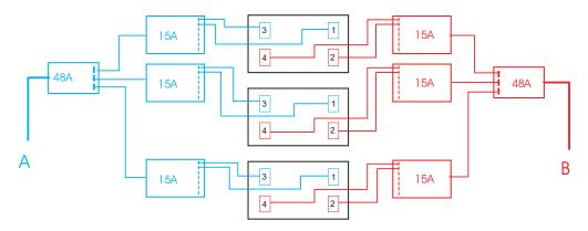
Figure 23. Three BladeCenter units in a NetBAY 25 or 42 rack; 1200 W power supplies
