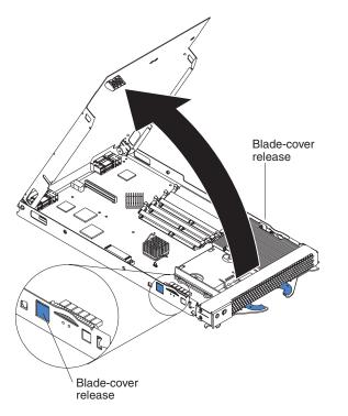
Figure 14. Opening the blade server cover
