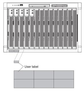
Figure 12. Applying a label to the BladeCenter Type 8677
