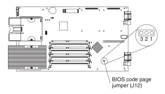
Figure 6. System board: BIOS code page jumper
