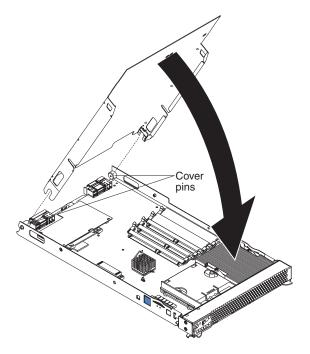
Figure 15. Closing the blade server cover
