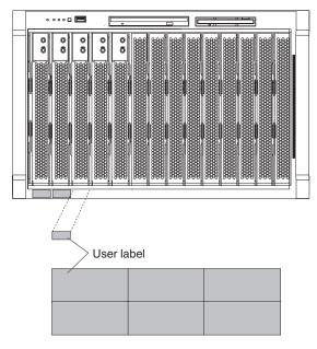
Figure 2. Label placement, Blade Center unit
