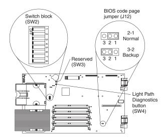
Figure 30. System board switches and jumpers
