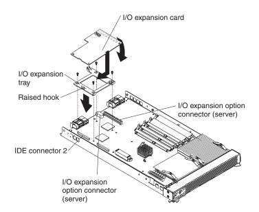
Figure 24. Installing an I/O expansion card
