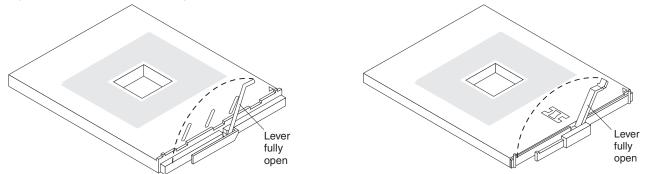
Figure 22. Microprocessor locking lever in the fully open position
