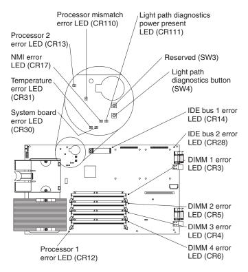
Figure 5. System board: light path diagnostics
