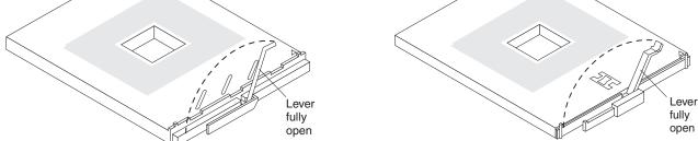
Figure 28. Microprocessor locking lever in the fully open position
