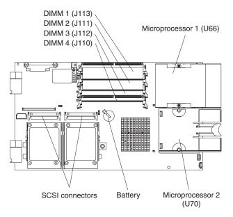
Figure 29. System board component locations
