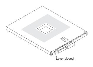
Figure 21. Microprocessor locking lever in the closed position
