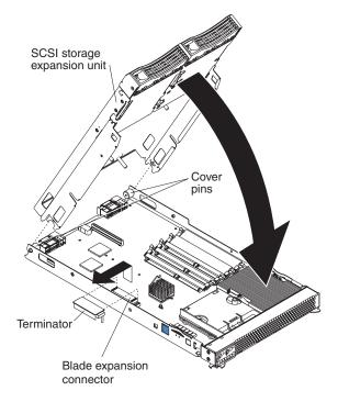
Figure 25. SCSI storage expansion unit installation
