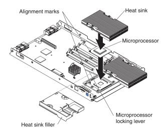
Figure 20. Installing a second microprocessor
