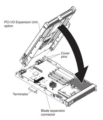
Figure 26. PCI I/O expansion unit installation
