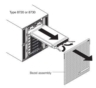
Figure 9. Blade server removal in the BladeCenter unit Type 8720 or 8730
