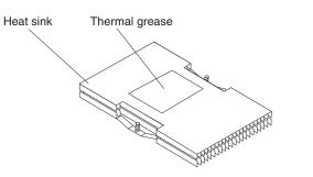
Figure 23. Location of thermal grease on heat sink
