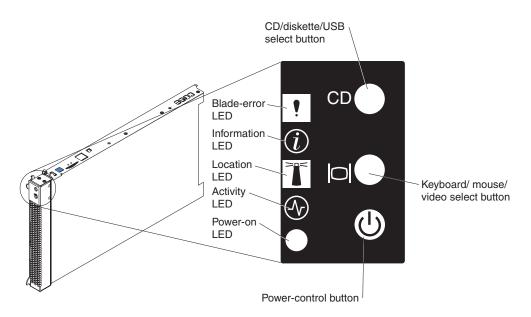
Figure 4. Controls and LEDs
