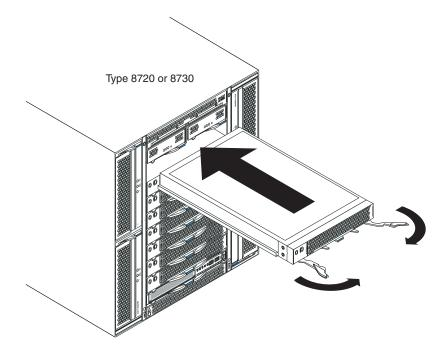
*Figure 11. Blade server installation in the BladeCenter unit Type 8720 or 8730* Complete the following steps to install a blade server in the BladeCenter unit:
