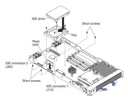
Figure 18. Installing an IDE drive
