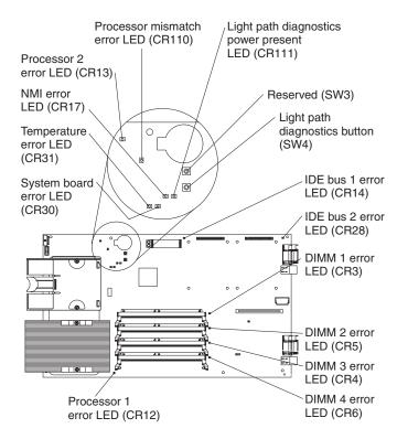
Figure 31. System board LED locations
