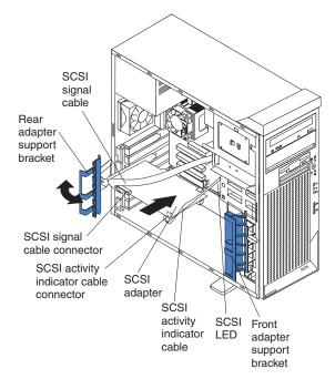
4. Complete the installation of the optional SCSI adapter.
