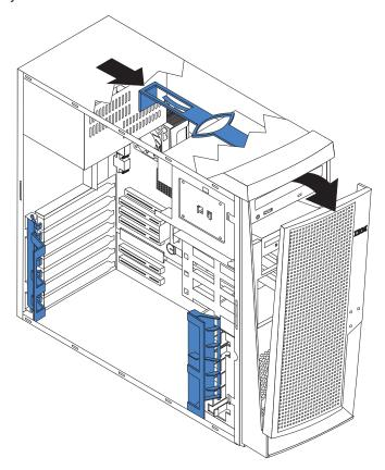
6. Pull the bezel up to release the two tabs at the bottom edge of the bezel. Store the bezel in a safe place.
