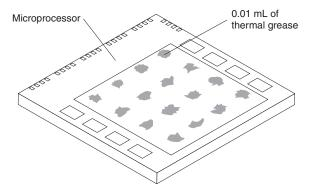
Use the thermal grease syringe to place 16 uniformly spaced dots of 0.01ML each on the top of the microprocessor.
