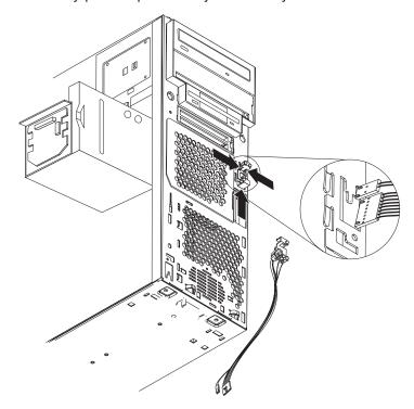
7. Note where the power-switch and LED panel cable connects to the system board; then, carefully disconnect the cable from the system board.
