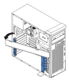
To reinstall the support bracket, reverse the previous steps.
