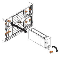
7. Attach any cables or cords required by the module. See "Input/output connectors" on page 60 for the location of connectors on the BladeCenter unit. Be sure to route the power cord on a power module through the strain-relief clamp on the power module.
