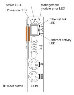
**Management-module LEDs:** These LEDs provide status information about the management module and remote-management connection. For additional information, see "Identifying problems using the Light Path Diagnostics feature" on page 43.
