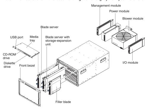
**Attention:** To maintain proper system cooling, each module bay must contain either a module or a filler module; each blade bay must contain either a blade server or a filler blade.
