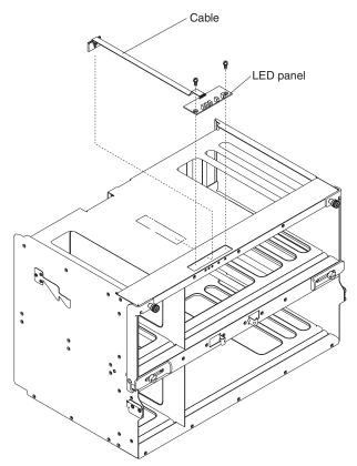
**Note:** You might need to push the LED panel cable toward the panel to leverage the panel out of the chassis opening.
