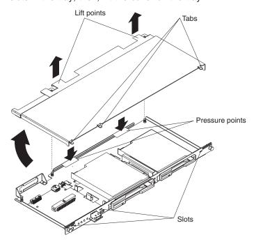
Reverse these instructions to reinstall the media tray cover. Press the rear of the cover down onto the two fasteners to secure the cover in place.
