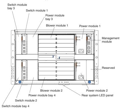
See "BladeCenter components, controls, and LEDs" on page 10 for details about these components and indicators.
