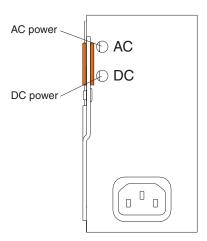
**Power module LEDs:** These green LEDs indicate the condition of the power module. For additional information, see "Identifying problems using the Light Path Diagnostics feature" on page 43.
