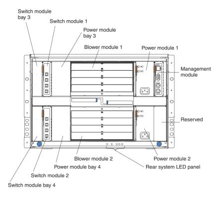
**Rear system LED panel:** The LEDs on this panel provide status information for your BladeCenter unit. These LEDs duplicate the LEDs in the front system LED panel, see "System LED panel" on page 15 for more information about these LEDs.
