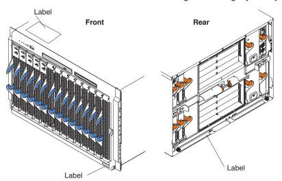
A set of user labels comes with each blade server. Write whatever identifying information you want on a label, and place it on the BladeCenter bezel just below the blade server, as shown in the following illustration.
