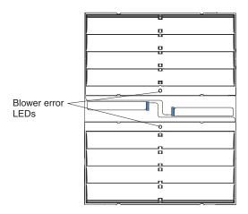
**Important:** If the ambient temperature is 72° F or below, the BladeCenter blowers will run at 30% of their maximum rotational speed, increasing their speed as required to control internal BladeCenter temperature. If ambient temperature is above 72° F, the blowers will run at 80% of their maximum rotational speed increasing their speed as required to control internal BladeCenter temperature.
