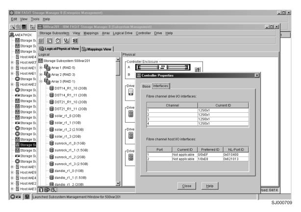
Figure 3. Controller Properties window
