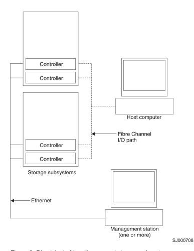
Figure 2. Direct (out-of-band) managed storage subsystems
