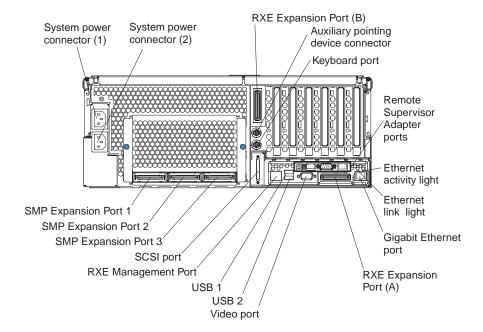
**System power connectors (1 and 2):** The system power cords are connected to these two connectors to provide power to the system.
