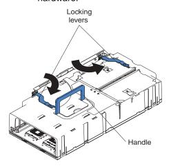
2. Install the SMP Expansion Module into the server.
