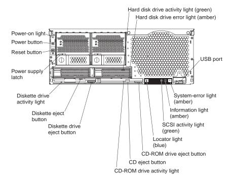
**Power-on light:** This green light turns on and stays on when you turn on your server, and it blinks when the server is in Standby mode.
