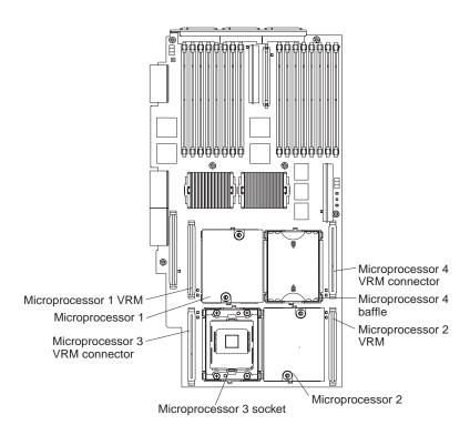
Complete the following steps to install a microprocessor:
