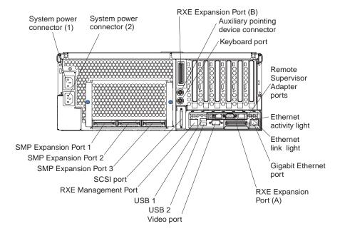
**System power connectors (1 and 2):** The system power cords are connected to these two connectors to provide power to the system.
