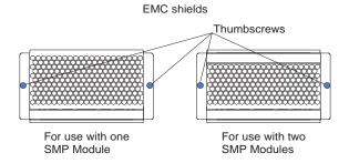
c. Remove the EMC shield from the rear of the server.
