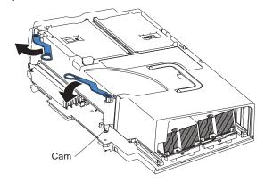
c. Using the locking levers, lift the front edge of the cover off the SMP Expansion Module.
