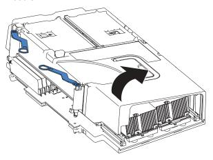
d. Lift the cover off the SMP Expansion Module.
