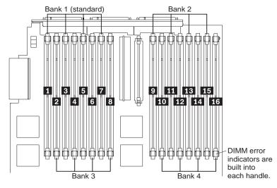
• Each DIMM in an individual bank must be of the same size and clock speed to ensure the server will operate properly.
