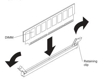
a. Open the retaining clip on each end of the DIMM connector. Turn the DIMM so that the pins align correctly with the connector.
