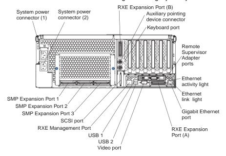
To effectively manage the cables on this server, keep groups of cables secured together, and do not run cables across the back of the server.
