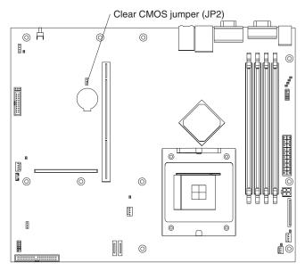
Complete the following steps to change the position of the clear CMOS jumper:
