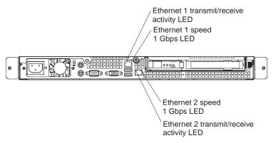
Ethernet 1 transmit/receive activity LED: This LED is on the Ethernet connector. When this LED is lit, it indicates that there is activity between the server and the network.
