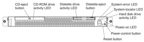
CD-eject button: Press this button to release a CD from the CD-ROM drive.
