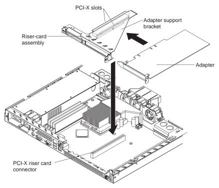
Complete the following steps to install an adapter:
