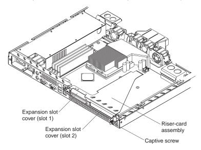
6. Remove the expansion-slot cover.
