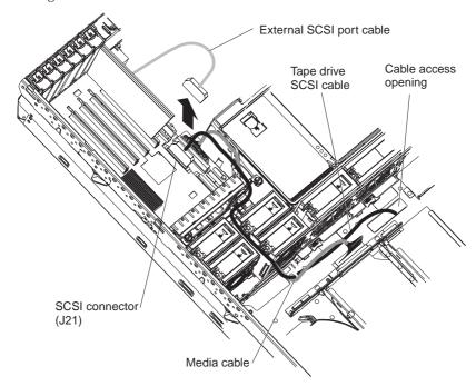
4. Route the tape drive SCSI cable through the cable access opening as shown in the illustration.
