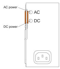
**Power module LEDs:** These green LEDs indicate the condition of the power module. For additional information, see the "Light Path Diagnostics" section in the BladeCenter *Hardware Maintenance Manual and Troubleshooting Guide* on the IBM *BladeCenter Documentation* CD.
