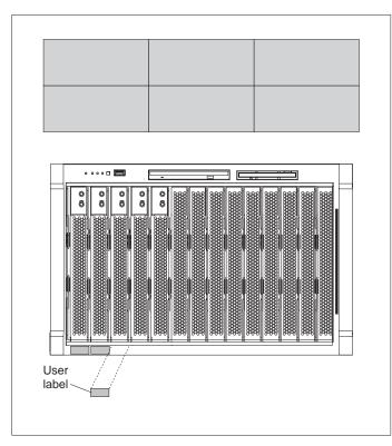
**Important:** Do not place the label on the blade server itself or in any way block the ventilation holes on the blade server.
