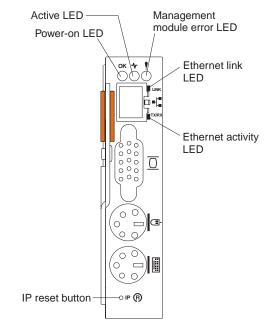
**Management module LEDs:** These LEDs provide status information about the management module and remote management connection. For additional information, see the "Light Path Diagnostics" section in the *Hardware Maintenance Manual and Troubleshooting Guide* on the IBM *BladeCenter Documentation* CD.
