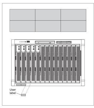
**Important:** Do not place the label on the blade server or in any way block the ventilation holes on the blade server.
