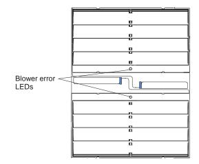
**Blower LEDs:** The LED on each blower provides status information about the blower. For additional information, see the "Light Path Diagnostics<sup>™</sup>," section in the BladeCenter *Hardware Maintenance Manual and Troubleshooting Guide* on the IBM *BladeCenter Documentation* CD.
