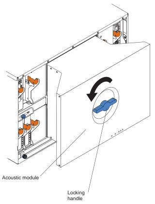
Complete the following steps to remove an acoustic module option from the BladeCenter unit:
