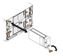
Complete the following steps to remove a power module, management module, or switch module. See the *Hardware Maintenance Manual and Troubleshooting Guide* on the *BladeCenter Documentation* CD for information about replacing a blower module.
