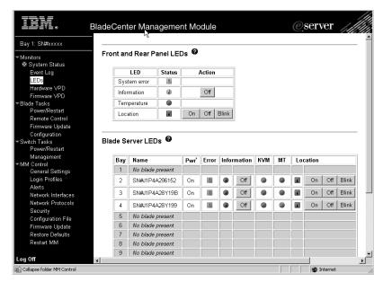
Select this choice to view the state of the BladeCenter system LED panel and blade server control panel LEDs. You also can use this choice to turn off the information LED and turn on, turn off, or blink the location LED on the BladeCenter unit and the blade servers.
