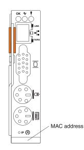
**Note:** If the IP configuration is assigned by the DHCP server, the network administrator can use the MAC address of the management module network interface to find out what IP address and host name are assigned.
