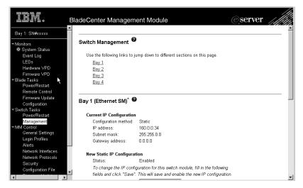
Select this choice to view or change the IP configuration of the Ethernet or Fibre Channel switch modules, ping a switch module, return a switch module to the default configuration, and start the configuration and management firmware that is in the switch module.
