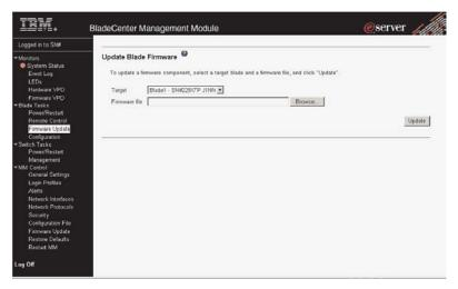
Select this choice to update the service processor firmware on a blade server. Select the target blade server and the firmware file to use for the update; then, click **Update**. You can obtain the firmware files from the IBM Support Web site at http://www.ibm.com/pc/support/.
