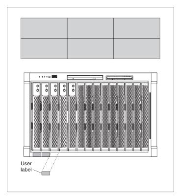
**Important:** Do not place the label on the blade server or in any way block the ventilation holes on the blade server.
