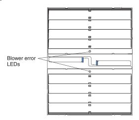
**Blower LEDs:** The LED on each blower provides status information about the blower. For additional information, see the "Light Path Diagnostics™" section in the BladeCenter *Hardware Maintenance Manual and Troubleshooting Guide* on the IBM *BladeCenter Documentation* CD.
