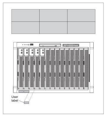
Important: Do not place the label on the blade server itself or in any way block the ventilation holes on the blade server.
