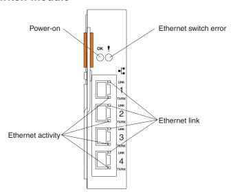
**Ethernet switch LEDs:** The LEDs on the switch module indicate the condition of the Ethernet switch and the links to the network. For additional information, see the "Light Path Diagnostics" section in the *Hardware Maintenance Manual and Troubleshooting Guide* on the IBM *BladeCenter Documentation* CD.
