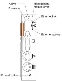
**Management module LEDs:** These LEDs provide status information about the management module and remote management connection. For additional information, see the "Light Path Diagnostics" section in the *Hardware Maintenance Manual and Troubleshooting Guide* on the IBM *BladeCenter Documentation* CD.
