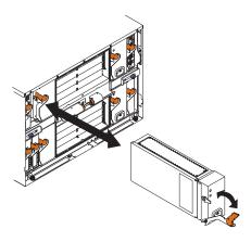
Complete the following steps to remove a power module, management module, or switch module. See the *Hardware Maintenance Manual and Troubleshooting Guide* on the *BladeCenter Documentation* CD for information about replacing a blower module.
