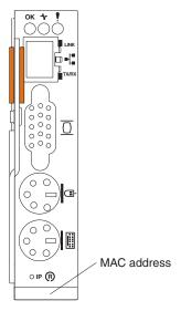
Important: Pressing the IP reset button on the management module replaces the configured IP addresses for the management module with the factory default IP addresses, and loses the connection with the remote management station, the switch modules, and the blade servers. If you press this button, you will need to reconfigure the management module settings.
