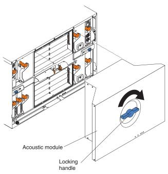
Complete the following steps to install an acoustic module option on the BladeCenter unit:
