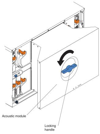
Complete the following steps to remove an acoustic module option from the BladeCenter unit:
