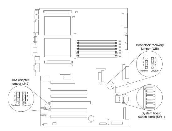
Table 2 describes the function of each switch on the switch block.
