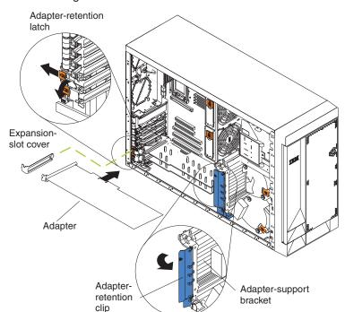
The following illustration shows how to install a PCI or PCI-X hot-plug adapter.
