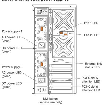
Fans 1 and 2 LEDs: These LEDs provide status information about rear fans 1 and 2. For additional information, see the section about the Light Path Diagnostics feature in the Hardware Maintenance Manual and Troubleshooting Guide on the IBM xSeries Documentation CD.
