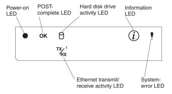
Important: If the power-on LED is off, it does not mean there is no electrical current present in the server. The LED might be burned out. To remove all electrical current from the server, you must unplug the server power cords from the electrical outlets or from the uninterruptible power
