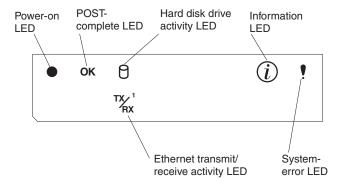
Important: If the power-on LED is off, it does not mean there is no electrical current present in the server. The LED might be burned out. To remove all electrical current from the server, you must unplug the server power cords from the electrical outlets or from the uninterruptible power device.
