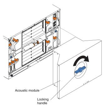
Complete the following steps to install an acoustic module option on the BladeCenter unit:
