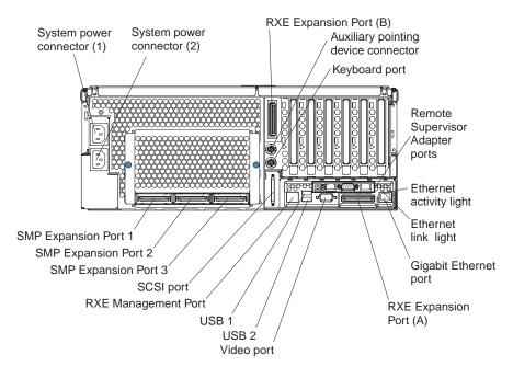
System power connectors (1 and 2): The system power cords are connected to these two connectors to provide power to the system.
