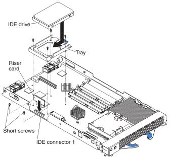
**Attention:** Do not press on the top of the hard disk drive. Pressing the top could damage the drive.
