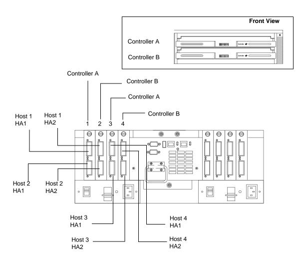
Figure 23. Connecting hosts directly to the controller
