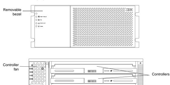
Figure 2. IBM FAStT500 RAID Controller Enclosure Unit – front view
