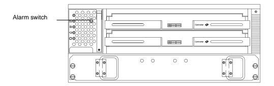
Figure 28. Controller unit alarm switch
