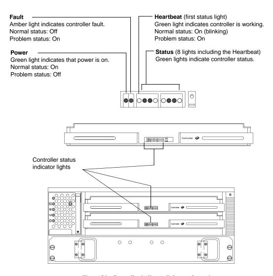
Figure 29. Controller indicator lights — front view
