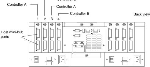
Figure 15. Controller unit host mini-hubs
