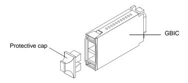
2 If the GBIC you are installing has a metal latch, move the latch to the unlocked (center) position. Slide the GBIC into the port; then, rotate the latch outward to the locked position (flush with the rear of the GBIC).
