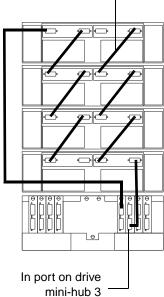
Figure 21. Cabling redundant drive enclosure loops to the controller unit
