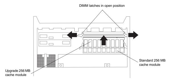
4 Carefully insert the DIMM into the empty socket, making sure that the left and right edges of the module slide inside the grooves in the DIMM latches. As you push the DIMM into place, the DIMM latches slowly close around the new module.
