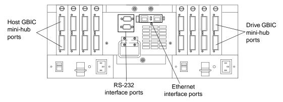
Figure 14. Controller unit interface ports
