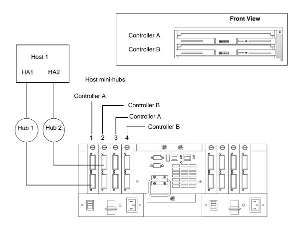
Figure 24. Using managed hubs to connect a host
