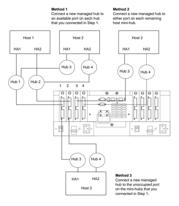
Figure 25. Using managed hubs to connect multiple hosts
