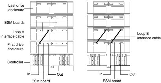
Figure 19. Example of connecting two drive enclosures into a redundant drive loop
