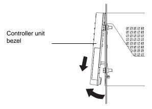
Figure 7. Removing the controller unit bezel
