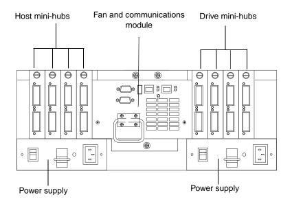
Figure 3. IBM FAStT500 RAID Controller Enclosure Unit – back view
