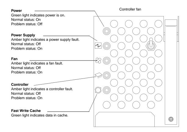
Figure 30. Controller fan indicator lights — front view
