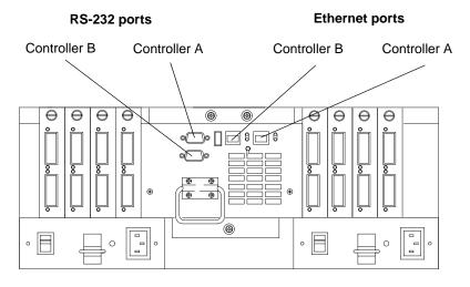
Figure 17. Controller unit Ethernet and RS-232 ports
