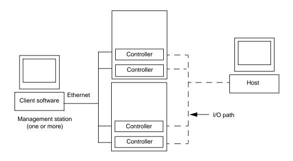
Figure 5. Direct-managed storage subsystems
