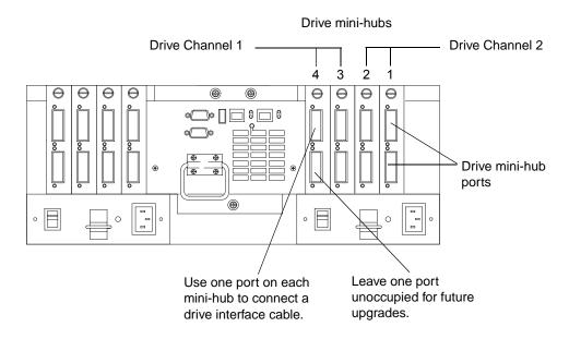
Figure 16. Controller unit drive mini-hubs
