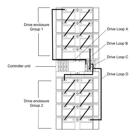
Figure 18. Redundant drive loop cabling overview
