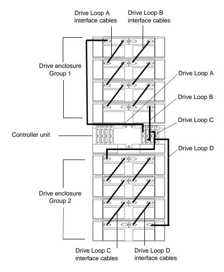
Figure 22. Two redundant drive enclosure groups
