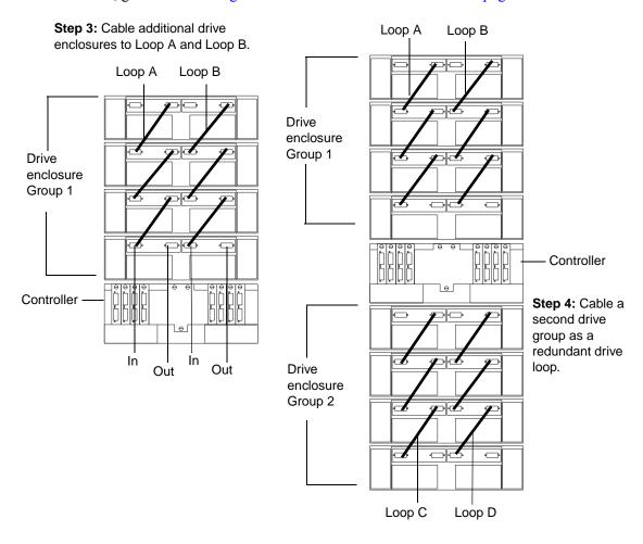
Figure 20. Connecting a second redundant drive loop
