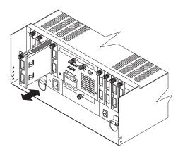
Figure 11. Removing and replacing the mini-hub
