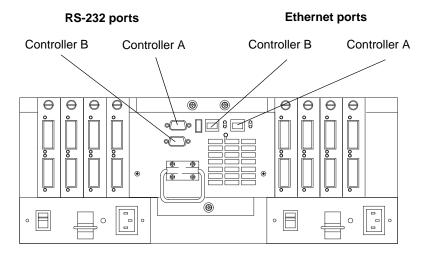
Figure 26. Connecting Ethernet and RS-232 interface cables
