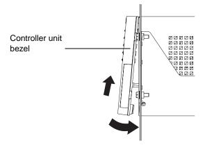
Figure 12. Replacing the controller unit bezel
