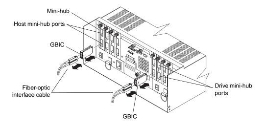
Figure 13. Mini-hub interface connections
