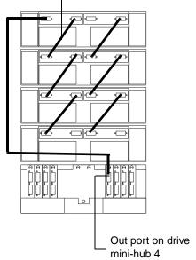
Step 2: Connect drive Loop B to the controller unit.
