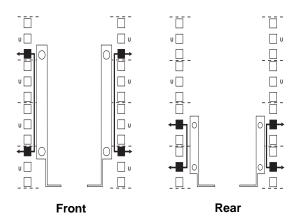
**Note:** Use clip nuts if your rack has round holes. If your rack has square holes, you can use the cage nut insertion tool or a flat-blade screwdriver to install cage nuts.
