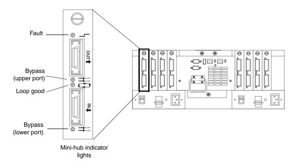
Figure 33. Mini-hub indicator lights
