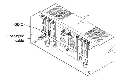
After you install the cables, the Fibre Channel Arbitrated Loop is operational.
