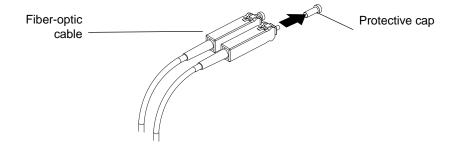
2 Connect the fiber-optic cable to a GBIC that is installed in a mini-hub.
