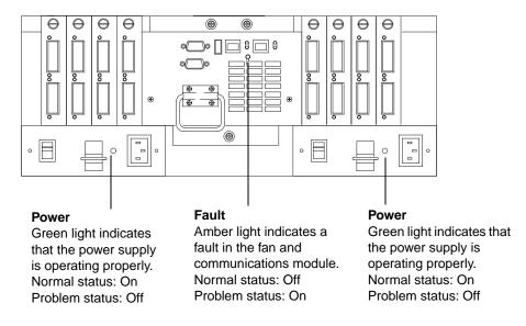
Figure 32. Controller unit indicator lights — back view
