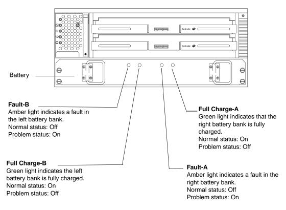
Figure 31. Battery indicator lights — front view
