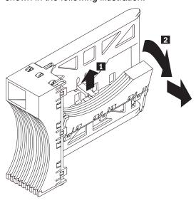
d. Insert the filler piece into the empty space that is left in the drive bay, as shown in the following illustration.
