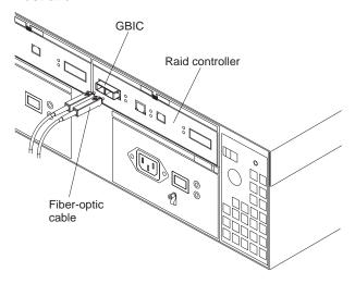
**Note:** The fiber-optic cable connection is keyed for proper insertion.
