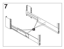
Tighten the rail adjustment screws 1 on both rails.
