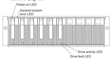
Figure 6. Storage server LEDs (front)
