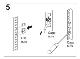
Use the attached template and stickers to mark the appropriate holes on your rack; then, install clip nuts or cage nuts as required for your rack cabinet.
