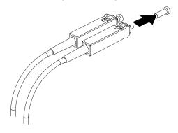
2. Connect the fiber-optic cable to the installed GBIC, as shown in the following illustration.
