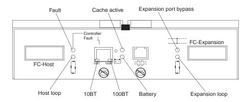
Figure 7. RAID controller LEDs
