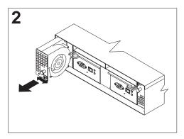
To remove a hot-swap fan, slide the latch on the fan to unlock it; then, pull the handle and remove the fan from the storage server.
