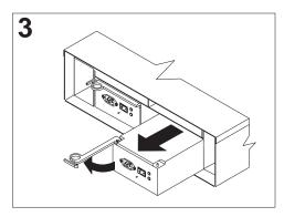
To remove a power supply, grasp the pull-ring on the power supply lever and squeeze to release it; then, pull the lever fully open and remove the power supply from the storage server.
