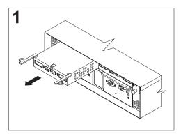
To remove a RAID controller, push down on the latch centered above the controller; then, grasp the pull-rings on the levers and pull them to remove the RAID controller and set it aside for later installation.
