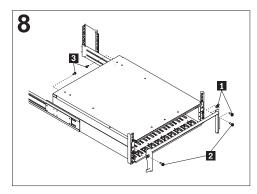
Remove the white screws and nuts 1 from the storage server bezel; then, slide the storage server into the rack. Align the bezel locator pins and attach the bezel with two M6 screws 2; then, install and tighten the 6-32 in. screws 3.
