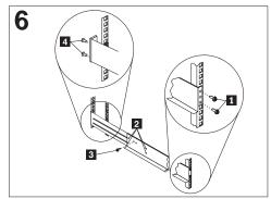
On the rail marked **R**, remove the 6-32 in. screw **3** and loosen the four screws **2**; then, hold the front of the rail against the outside of the right rack-mounting-flange and loosely install two M6 screws **1**.
