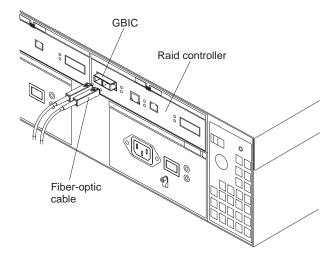
3. Check the LEDs on the RAID controller. When the RAID controller is operating properly, the amber Fault LED is off. For information about the status of the RAID controller LEDs, see Table 4 on page 30.
