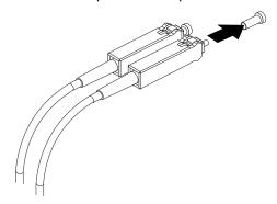
9. Connect the fiber-optic cable to the installed GBIC, as shown in the following illustration.
