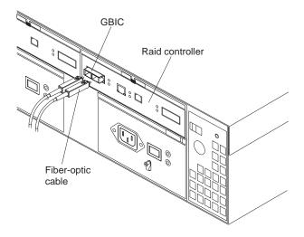
After removing the Fibre Channel cables, insert the protective caps.
