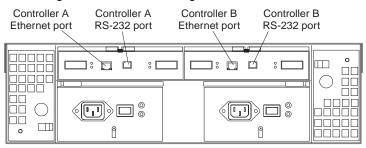
**Note:** The serial (RS-232) interface ports are intended to be used by service technicians to perform diagnostic operations on the storage server.
