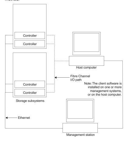
Figure 2. Direct-managed storage subsystems
