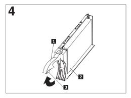
To remove a hard disk drive 2, press the blue latch 3 and pull the handle 1 upwards; then, carefully pull the drive from the storage server.
