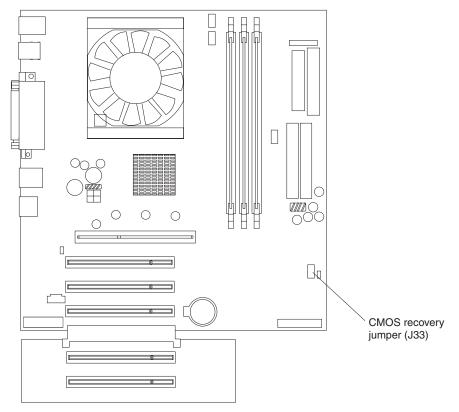
The CMOS recovery jumper can be used to clear CMOS memory in the event you lose your user password. See "Erasing a lost or forgotten password (clearing CMOS)" on page 109 for information about how to use the CMOS jumper.
