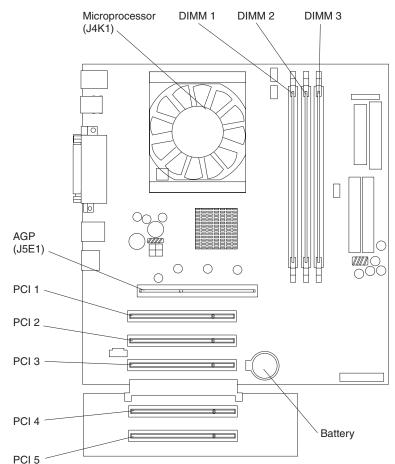
The following illustration shows the location of expansion slots on the system board.
