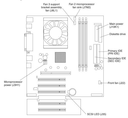
**System board external connectors**The following illustration identifies system board connectors for external cables.
