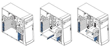
9. Connect the power and signal cables to the rear of each drive.
