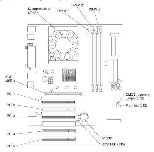
**System board internal cable connectors**The following illustration identifies system board connectors for internal cables.
