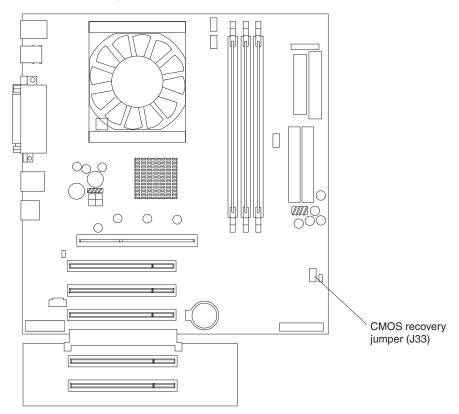
6. Move the jumper from pins 1 and 2 to the maintenance, or configure position (pins 2 and 3).
