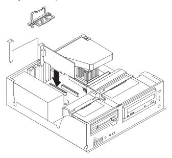
**Attention:** Be certain that the adapter is correctly seated in the expansion slot before you turn on the computer. Incomplete installation of an adapter might damage the system board or the adapter.
