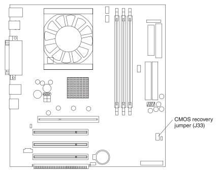
The CMOS recovery jumper can be used to clear CMOS memory in the event you lose your user password. See "Erasing a lost or forgotten password (clearing CMOS)" on page 109 for information about how to use the CMOS recovery jumper.
