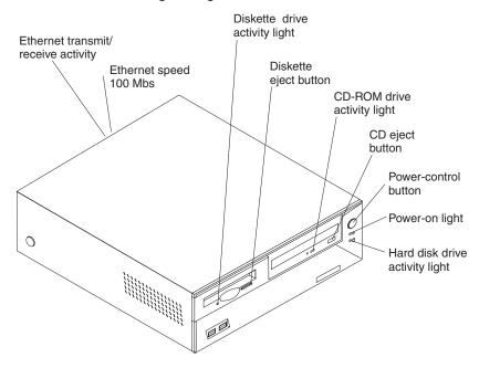
Note: The front bezel door is not shown here so that the drive bays are visible.
